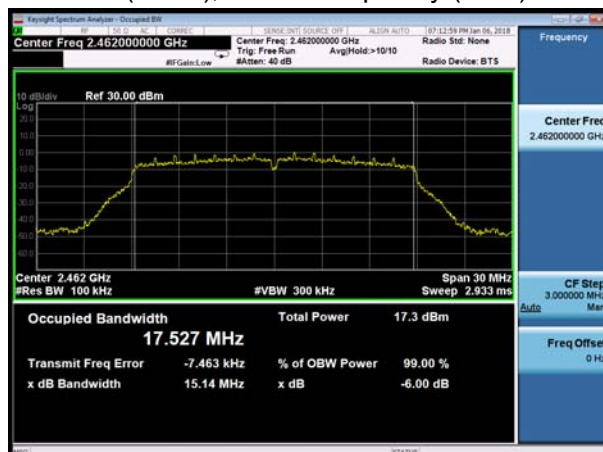
802.11n(HT20), Carrier frequency (MHz): 2462
