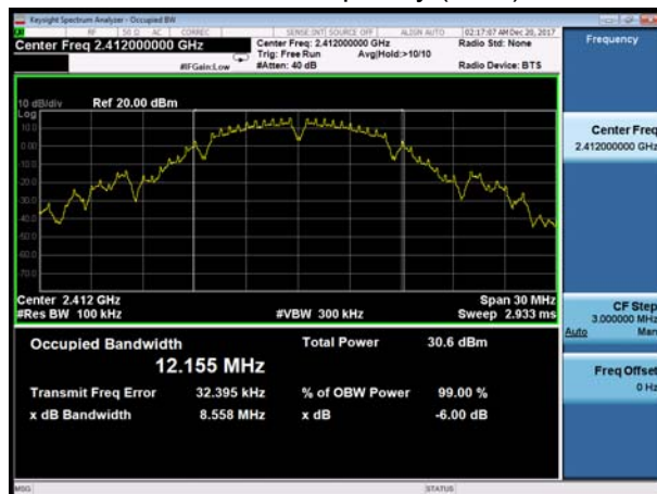
802.11b, Carrier frequency (MHz): 2437
