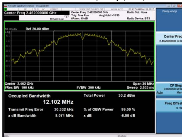
802.11b, Carrier frequency (MHz): 2462
