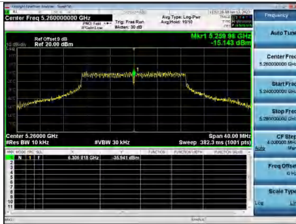
Freq. Stability 20C 120V ac20 5260MHz Ant1 0 Minutes
