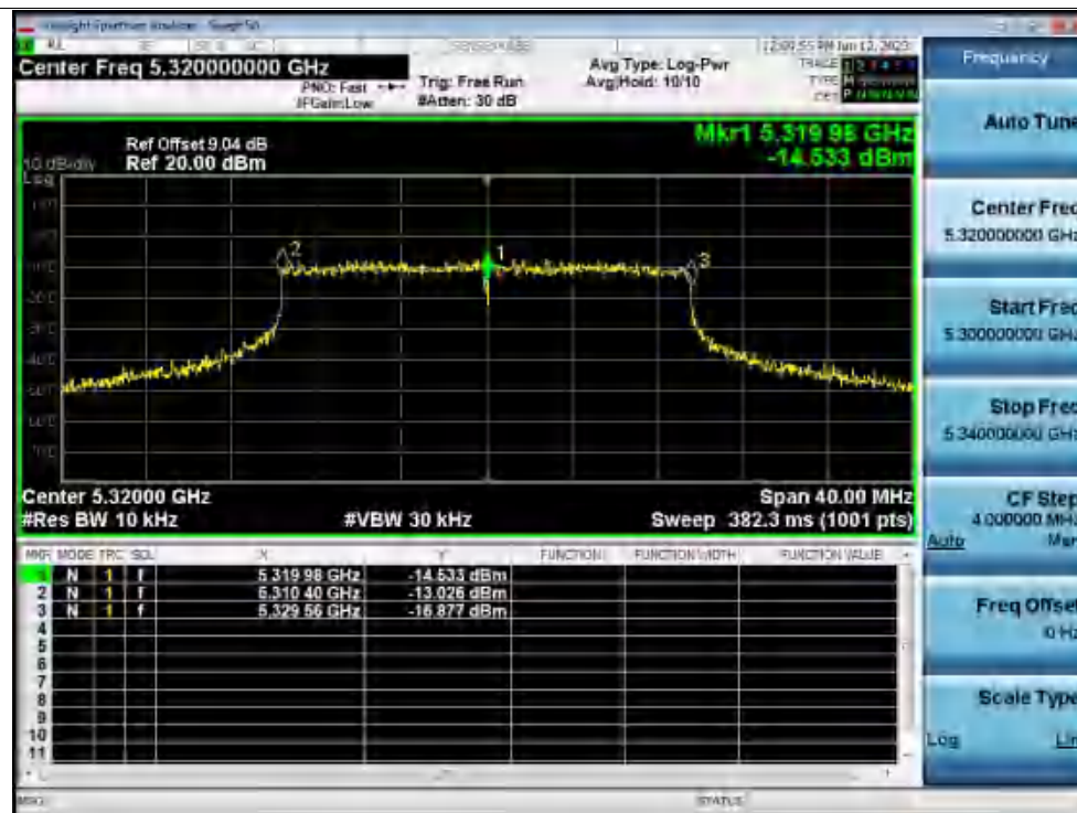
Freq. Stability 50C 120V ax20 5320MHz Ant1 0 Minutes
