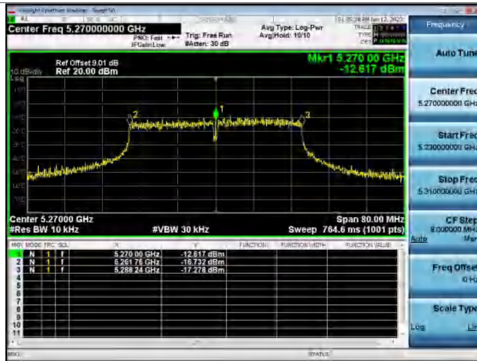
Freq. Stability 30C 120V ac40 5270MHz Ant1 0 Minutes
