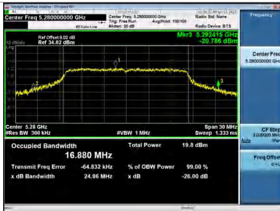
-26dB Bandwidth NVNT a 5280MHz Ant1
