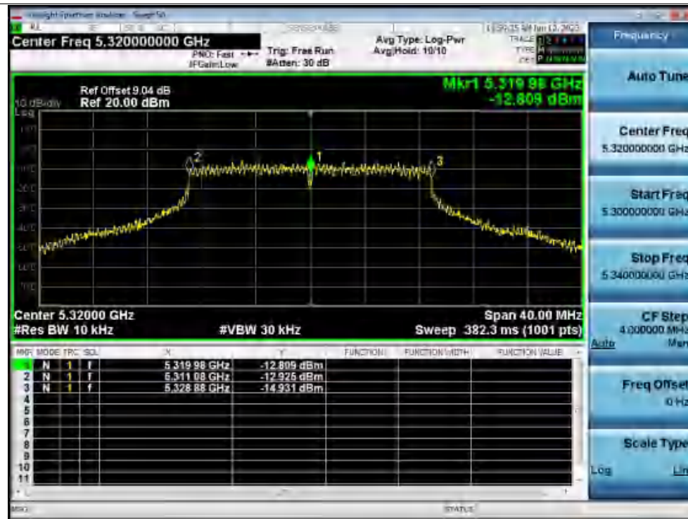
Freq. Stability 20C 120V ac20 5320MHz Ant1 0 Minutes
