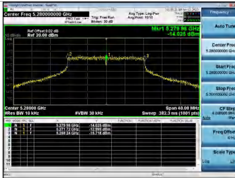
Freq. Stability 50C 120V a 5280MHz Ant1 0 Minutes
