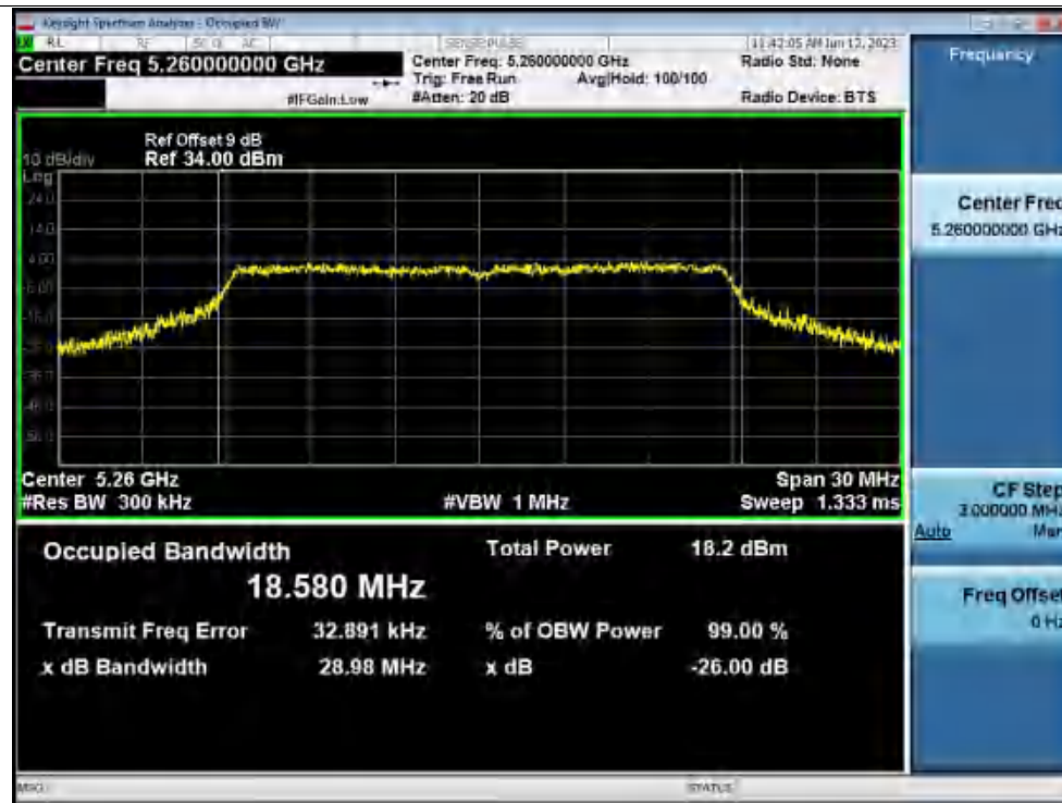
-26dB Bandwidth NVNT n20 5260MHz Ant1
