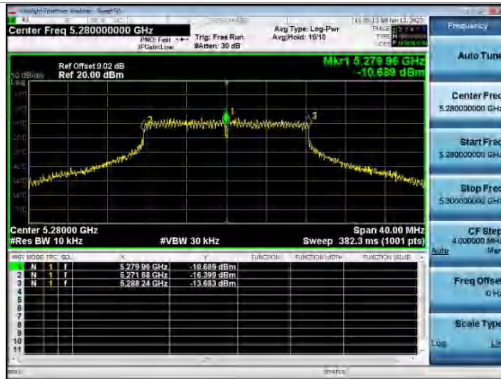
Freq. Stability 30C 120V a 5280MHz Ant1 0 Minutes
