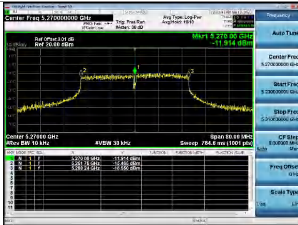
Freq. Stability 50C 120V n40 5270MHz Ant1 0 Minutes
