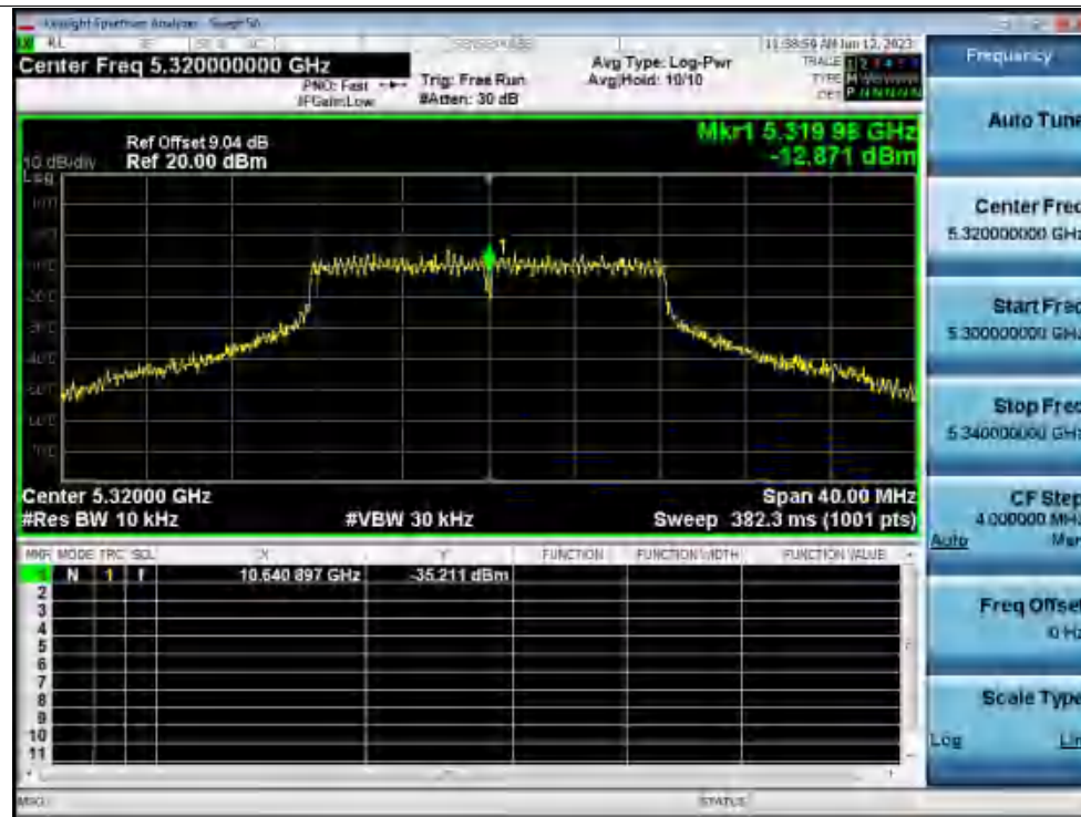
Freq. Stability 20C 120V a 5320MHz Ant1 0 Minutes
