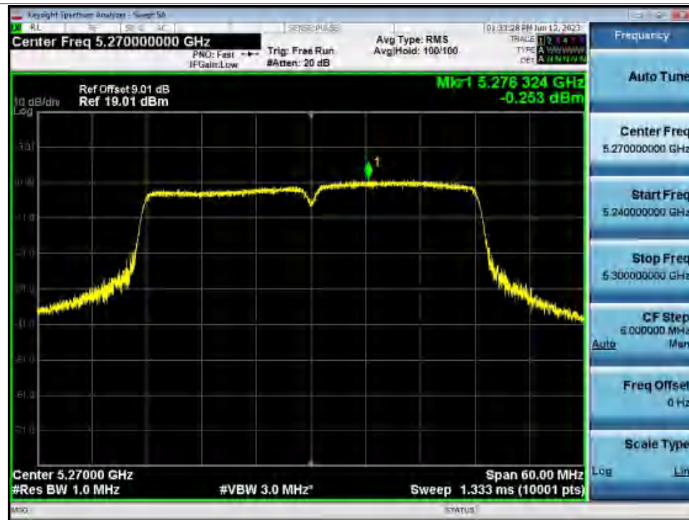
PSD NVNT ac40 5270MHz Ant1
