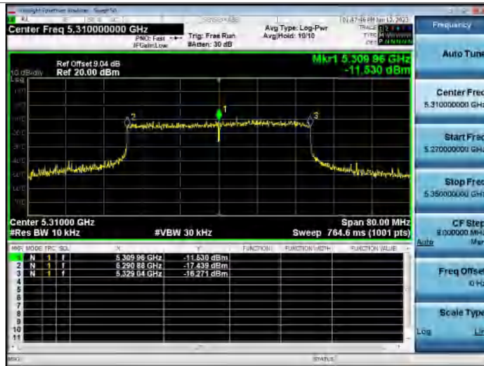
Freq. Stability 0C 120V ax40 5310MHz Ant1 0 Minutes
