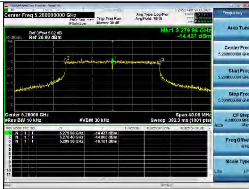
Freq. Stability 0C 120V ax20 5280MHz Ant1 0 Minutes
