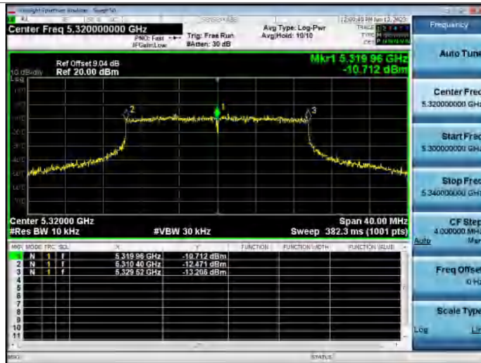
Freq. Stability 50C 120V ax20 5320MHz Ant1 0 Minutes
