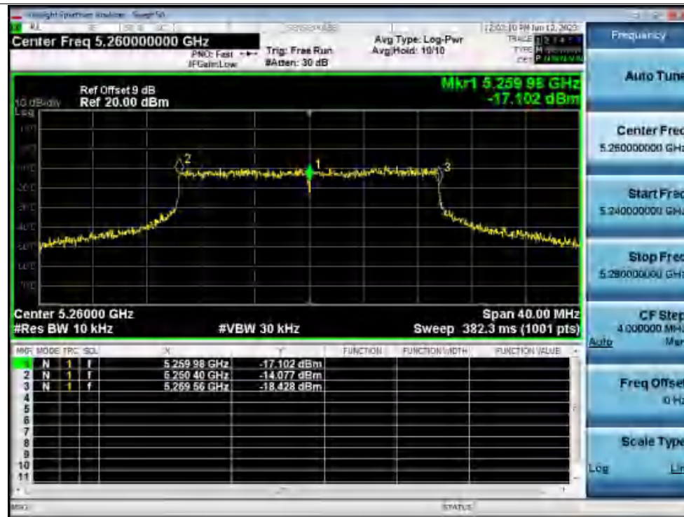
Freq. Stability -20C 120V ax20 5260MHz Ant1 0 Minutes
