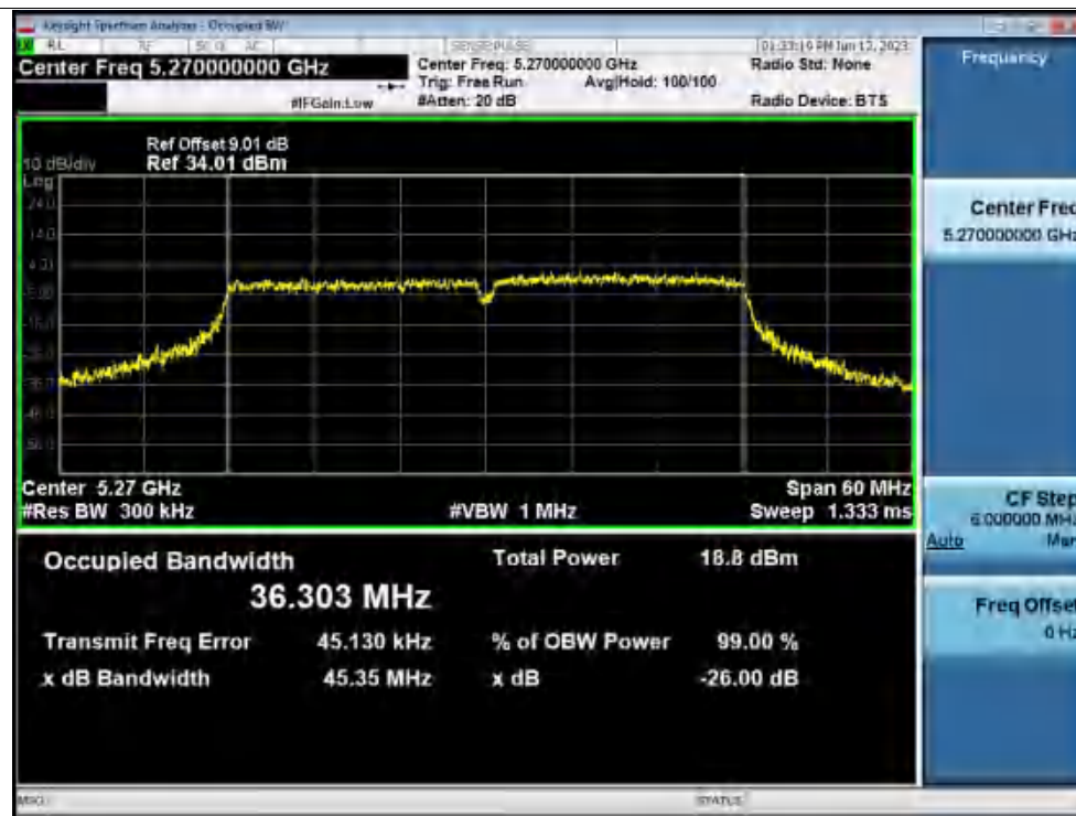
-26dB Bandwidth NVNT ac40 5270MHz Ant1
