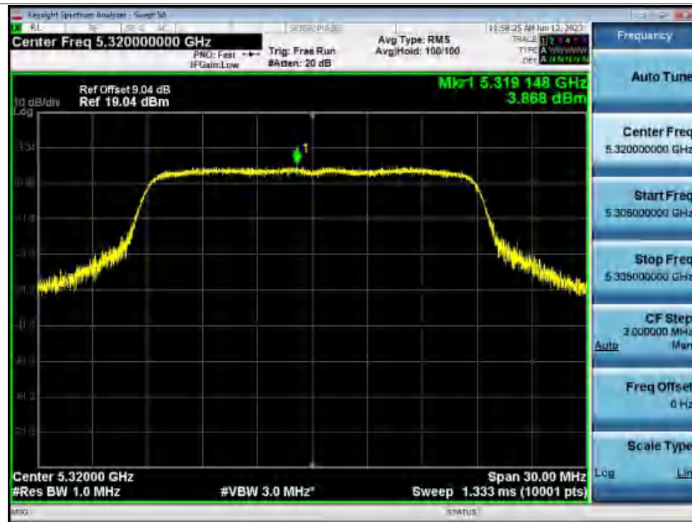
PSD NVNT ac40 5270MHz Ant1
