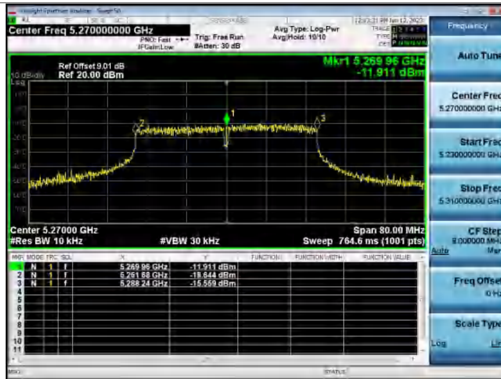
Freq. Stability 30C 120V n40 5270MHz Ant1 0 Minutes
