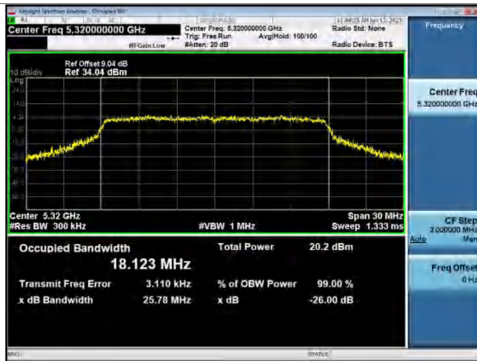
-26dB Bandwidth NVNT n20 5320MHz Ant1
