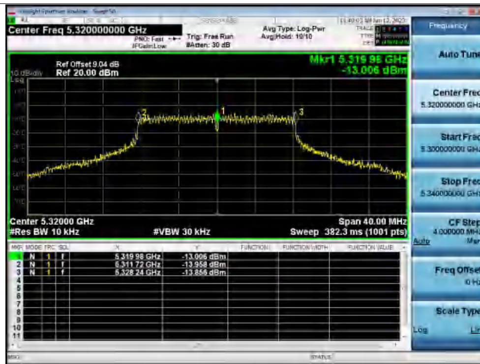
Freq. Stability 50C 120V a 5320MHz Ant1 0 Minutes
