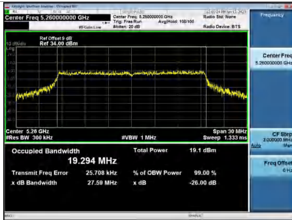
-26dB Bandwidth NVNT ax20 5280MHz Ant1
