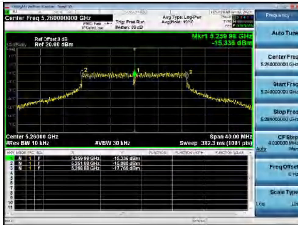
Freq. Stability 30C 120V ac20 5260MHz Ant1 0 Minutes
