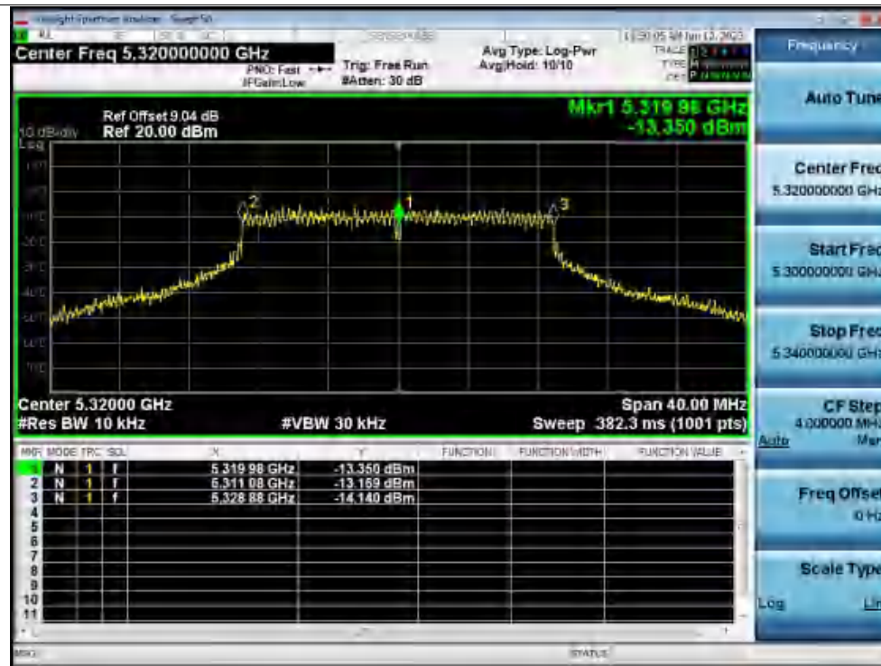
Freq. Stability 50C 120V n20 5320MHz Ant1 0 Minutes
