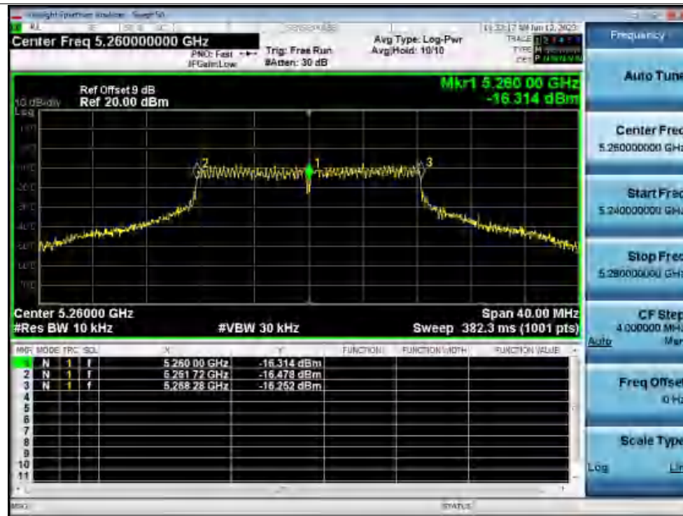
Freq. Stability 30C 120V a 5260MHz Ant1 0 Minutes
