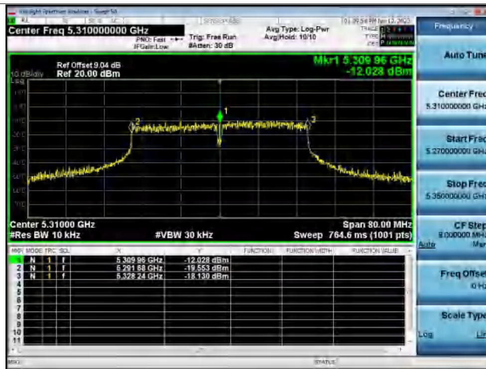
Freq. Stability 50C 120V ac40 5310MHz Ant1 0 Minutes
