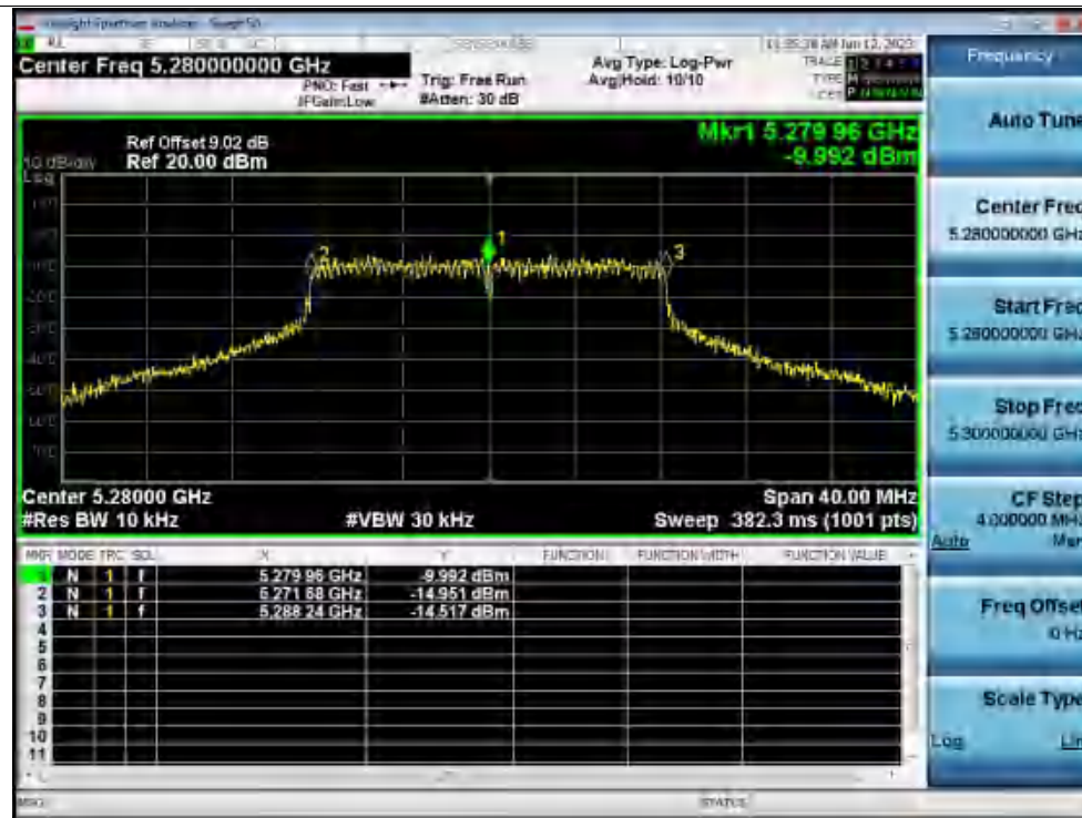
Freq. Stability 50C 120V a 5280MHz Ant1 0 Minutes
