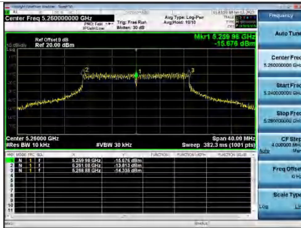
Freq. Stability -20C 120V n20 5260MHz Ant1 0 Minutes
