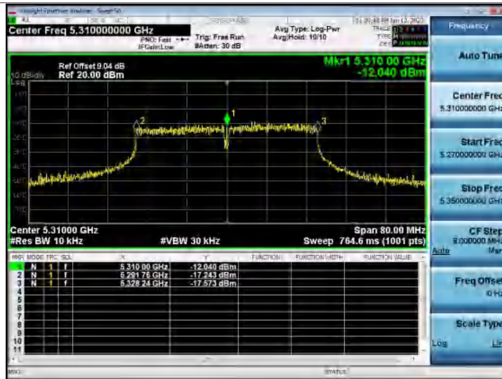
Freq. Stability 50C 120V ac40 5310MHz Ant1 0 Minutes
