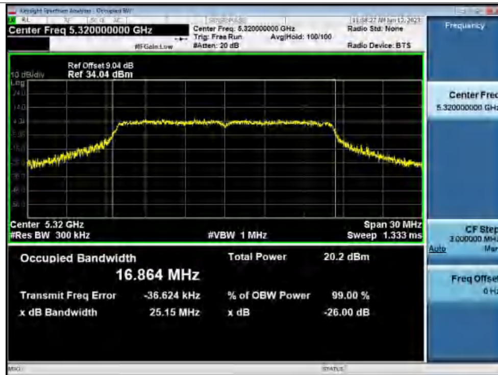
-26dB Bandwidth NVNT n20 5260MHz Ant1
