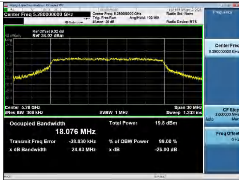
-26dB Bandwidth NVNT n20 5320MHz Ant1
