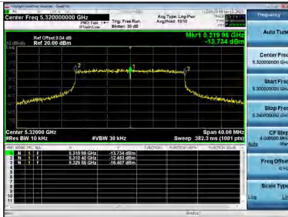
Freq. Stability 30C 120V ax20 5320MHz Ant1 0 Minutes
