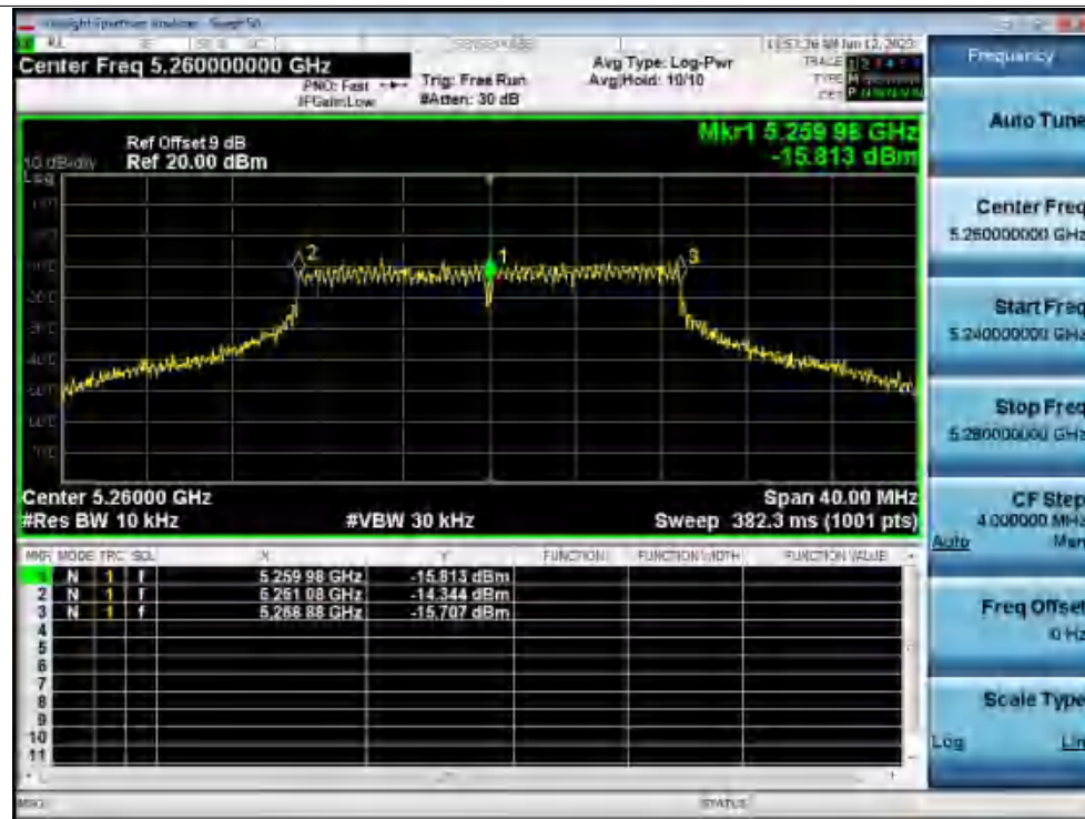
Freq. Stability 50C 120V ac20 5260MHz Ant1 0 Minutes
