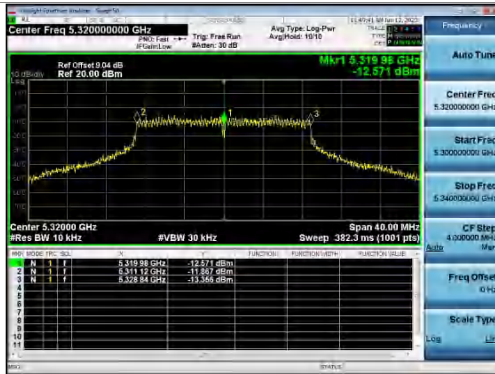
Freq. Stability 0C 120V n20 5320MHz Ant1 0 Minutes
