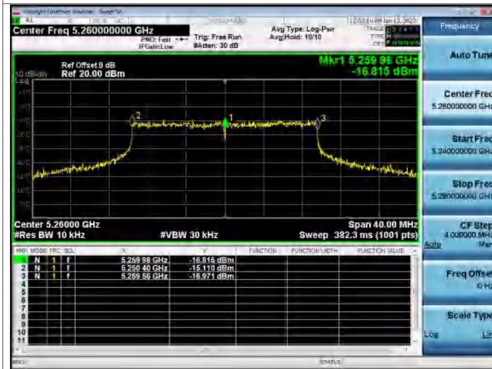
Freq. Stability -20C 120V ax20 5260MHz Ant1 0 Minutes
