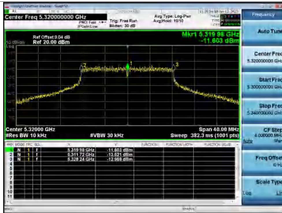
Freq. Stability 50C 120V a 5320MHz Ant1 0 Minutes
