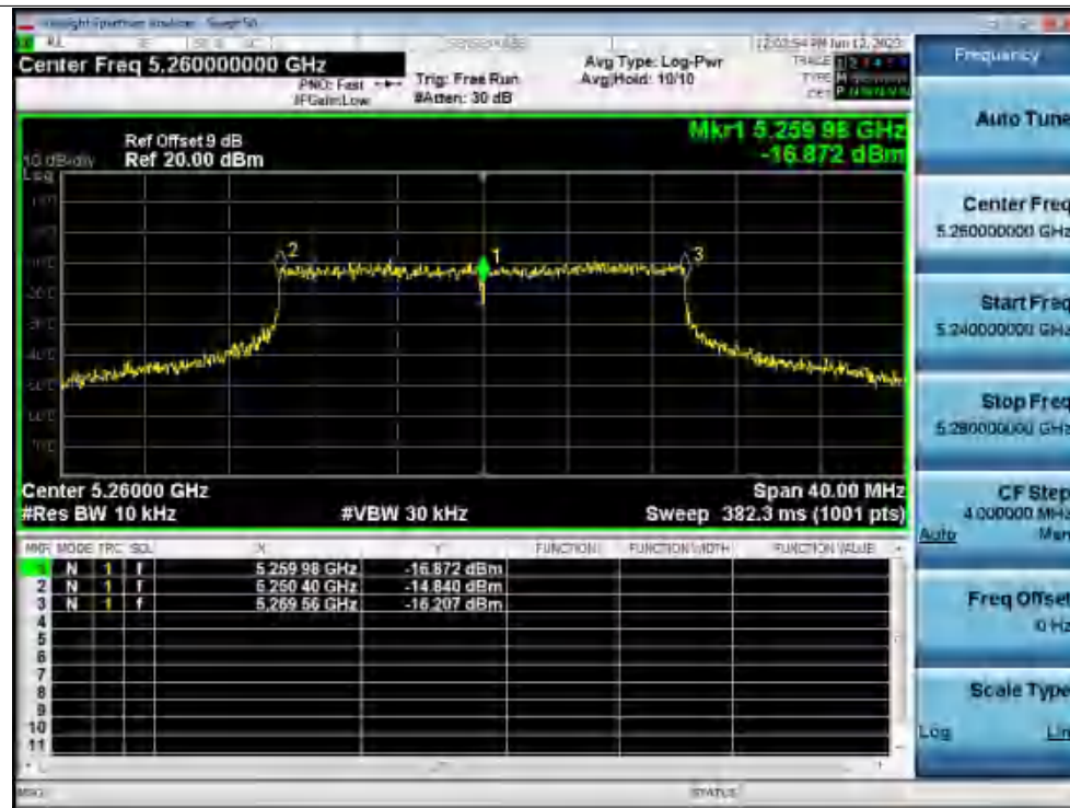
Freq. Stability 50C 120V ax20 5260MHz Ant1 0 Minutes
