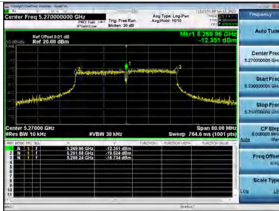
Freq. Stability 50C 120V n40 5270MHz Ant1 0 Minutes
