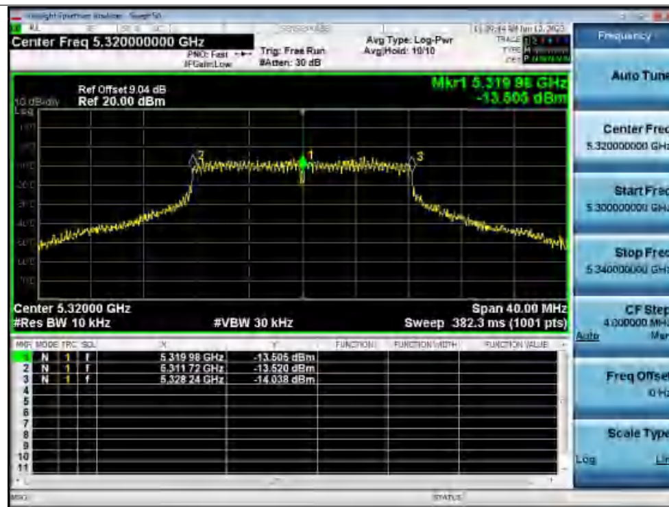
Freq. Stability 20C 120V a 5320MHz Ant1 0 Minutes
