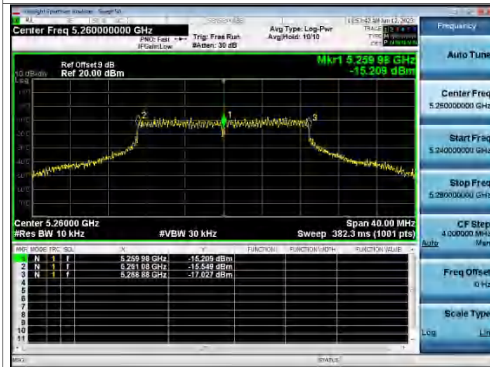
Freq. Stability 50C 120V ac20 5260MHz Ant1 0 Minutes
