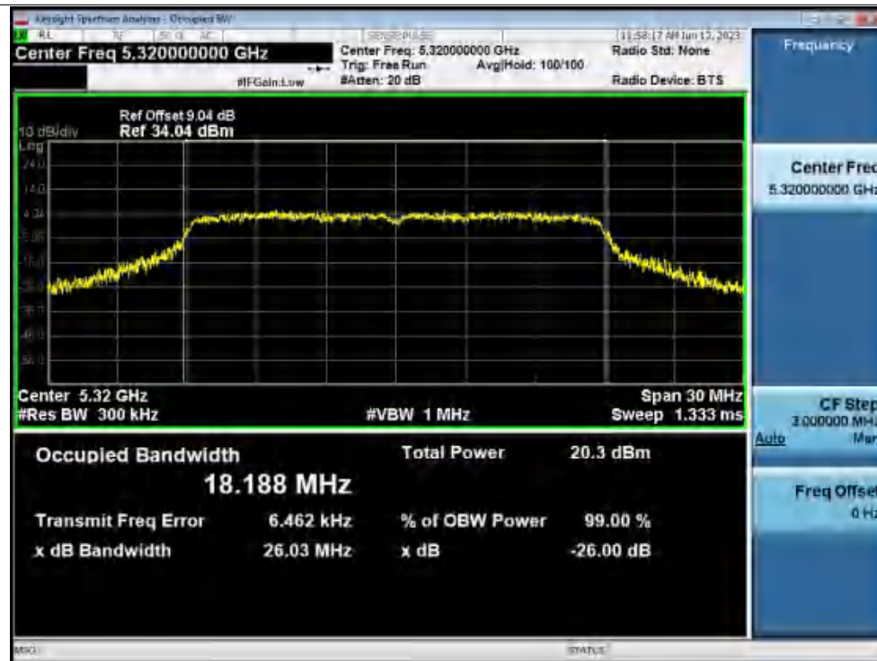
-26dB Bandwidth NVNT ac40 5270MHz Ant1
