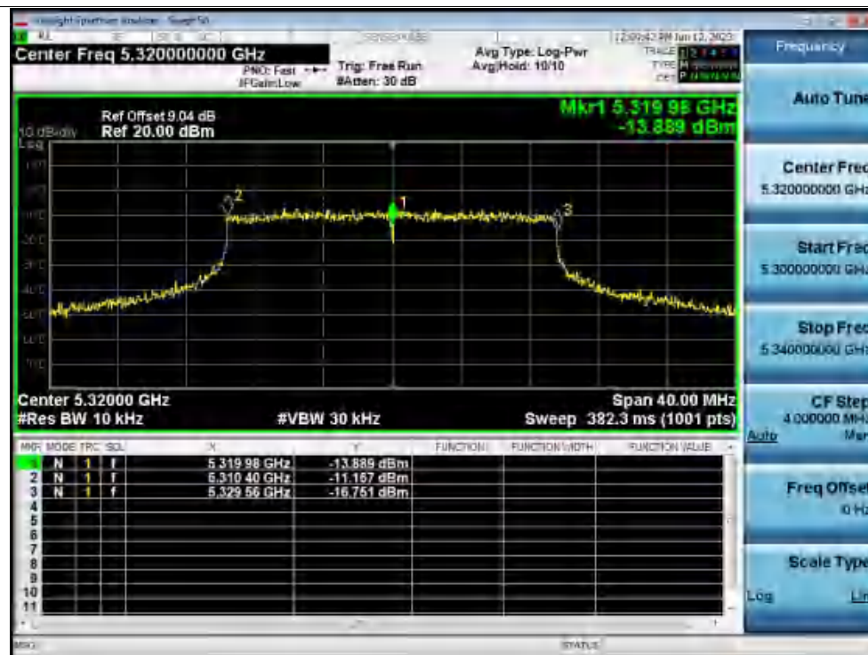
Freq. Stability 30C 120V ax20 5320MHz Ant1 0 Minutes
