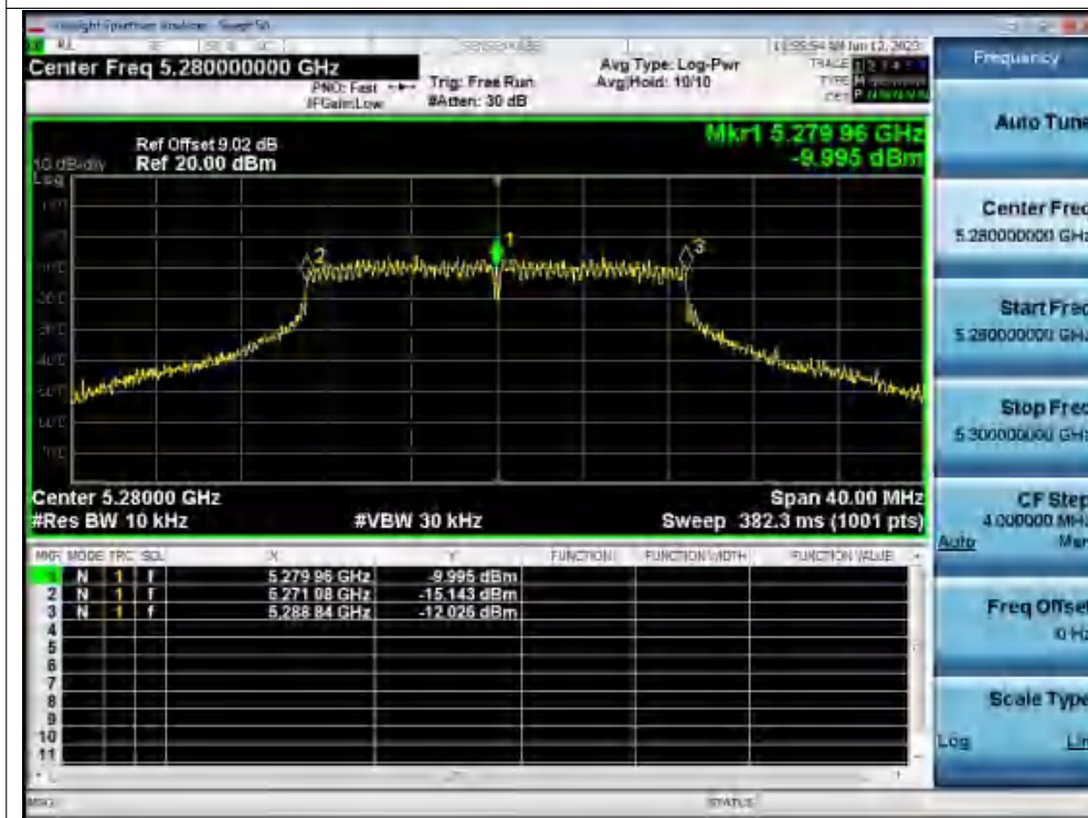
Freq. Stability -20C 120V ac20 5280MHz Ant1 0 Minutes
