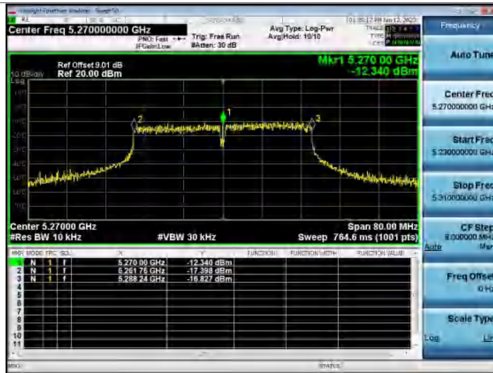
Freq. Stability 30C 120V ac40 5270MHz Ant1 0 Minutes
