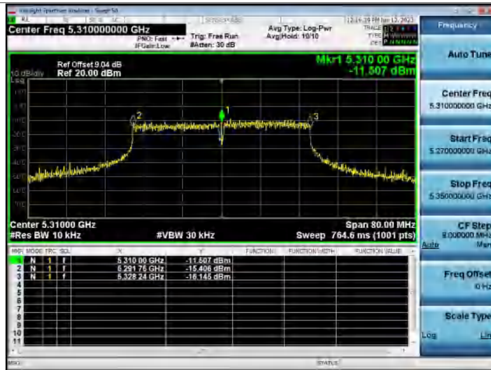
Freq. Stability 0C 120V n40 5310MHz Ant1 0 Minutes
