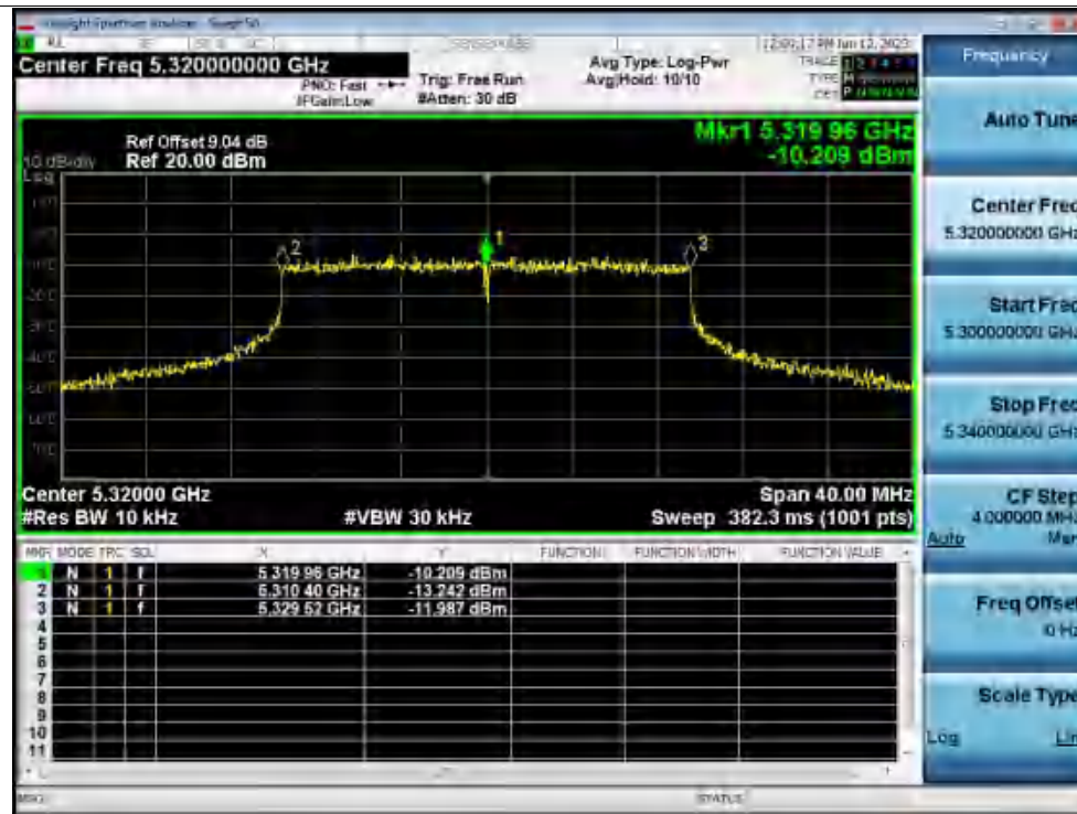
Freq. Stability 0C 120V ax20 5320MHz Ant1 0 Minutes
