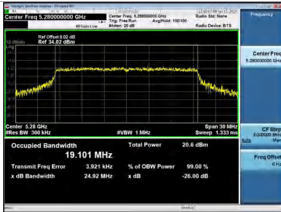
-26dB Bandwidth NVNT ax20 5280MHz Ant1
