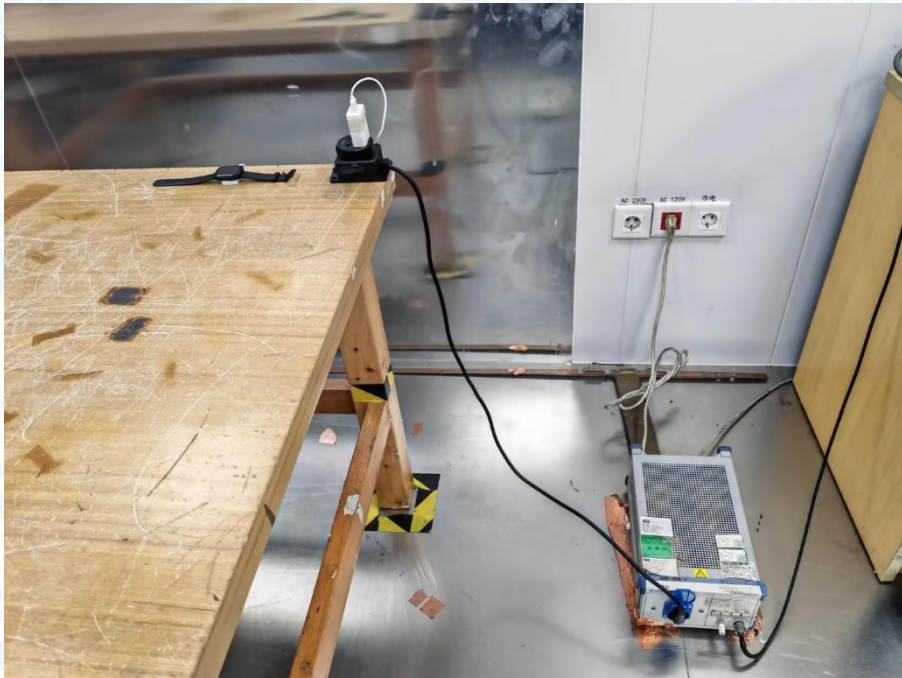
Photo of Setup for Radiated Emission (30MHz~1GHz)
