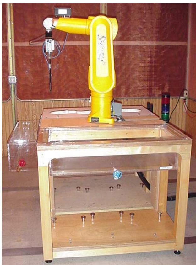
DASY4 SAR Measurement System with validation phantom
