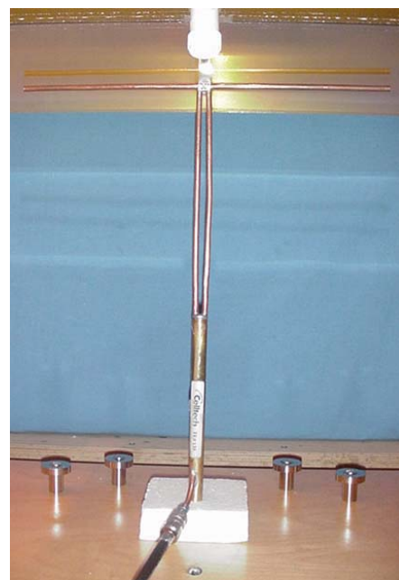
300 MHz Dipole Setup
