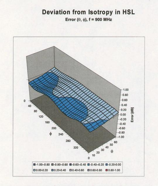
Spherical Isotropy Error < ± 0.4 dB
