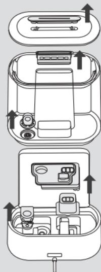
Remove the nozzle, droplet collector, cartridge, hot/cold mist mixer, noise silencer, and float.
