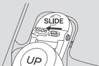
Fix the left prong on the bracket, then slide the other prong to secure the float in place.
