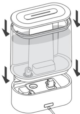
Put the water tank back in place and close the top cover.
