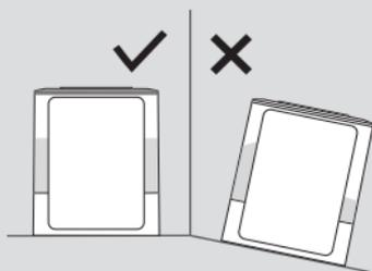
Make sure the humidifier is placed on a flat surface.
