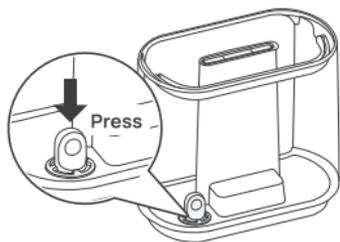
Place the cartridge back into the tank. Make sure the cartridge clicks in place.
