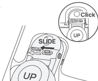
Fix the left prong on the bracket, then slide the other prong to secure the float in place.
