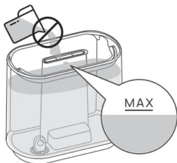
Fill the tank with water, making sure the water doesn't pass the MAX line.
