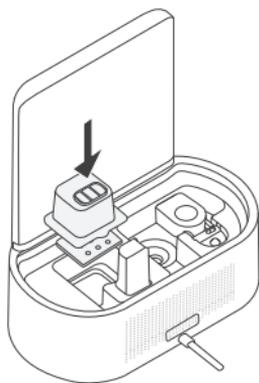
Place the absorption pad and the noise silencer back to the PTC heater.
