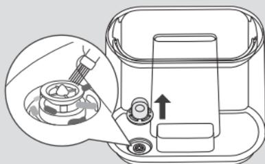
Remove any particles or hair blocking the water valve.
