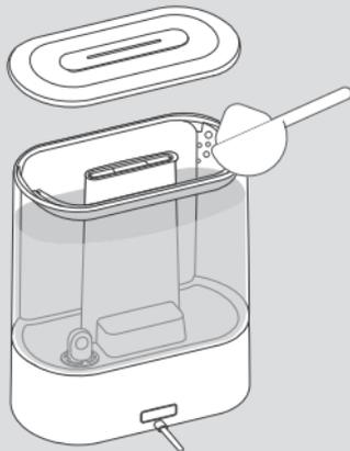
Fill the tank with a solution of citric acid and water (one teaspoon of citric acid for each gallon of water). Replace the tank cover and shake around the tank.
