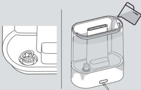
The water valve is not flat or the tank leaks water when refilling.
