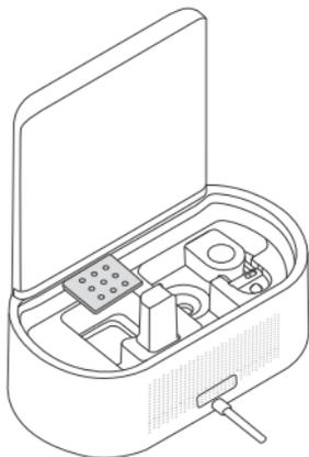
The mineral absorption pads help reduce mineral buildup (scale) inside the humidifier, especially on the heating element.
