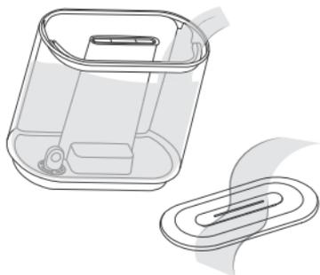
Detach the cover and water tank from the humidifier and clean thoroughly.
