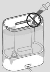
Your water tank has leakage due to prolonged use of essential oils.
