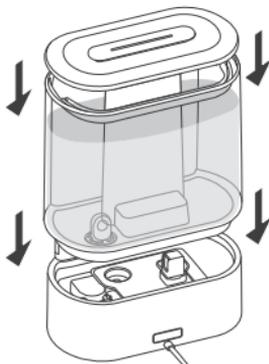
Attach the water tank to the base, replace the top cover.
