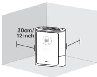
Place the humidifier on a flat, level surface, keeping at least 30 cm/ 12 inch away from walls or any major obstacles.
