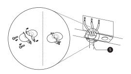
For conduit installations, insert the conduit strain relief in the 1 1/8 in. (2.8 cm) conduit hole. Then install the conduit through the body of the strain relief and fasten the strain relief with its ring.
