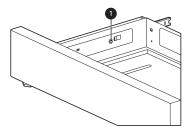
Locate the glide lever on each side of the drawer. Push down on the left glide lever and pull up on the right glide lever.
