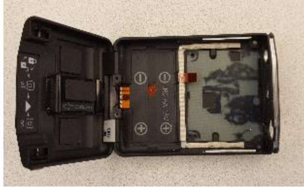
ULXD1 V50 Open Case, Circuit Board Removed
