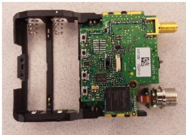
ULXD1 V50 Circuit Board Bottom
