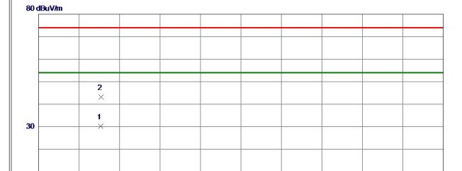
Measure Reading Correct No. Freq. Limit Margin Level Factor ment MHz dBuV/m dBuV/m dBuV/m dB Comment dB  ${\tt Detector}$ 1 \* 4922. 3800 24. 94 5.23 30.17 54.00 -23.83 AVG 4926. 3230 37. 93 5.25 43. 18 74.00 -30.82Peak
