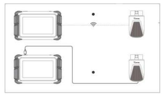
Note: The VCI box connects to the Diagnostic Tool via WiFi. If the WiFi function is not working currently, you can also connect to the Diagnostic Tool directly via a Type-C cable.
