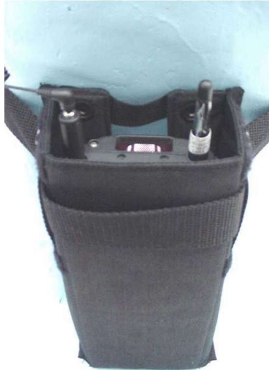
Back Side of DUT facing body - worst-case antenna configuration in relation to left arm
