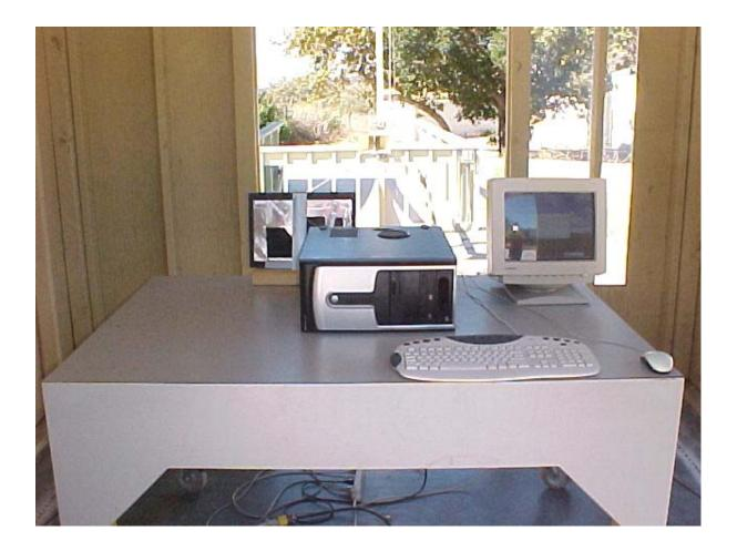
Radiated Emissions Measurement (Front View) Setup
