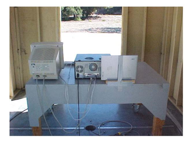
Radiated Emissions Measurement (Rear View) Setup
