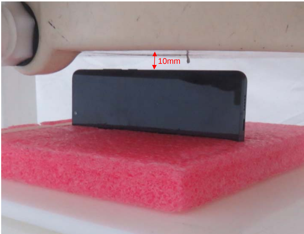
Picture 10: Right Side, the distance from handset to the bottom of the Phantom is 10mm
