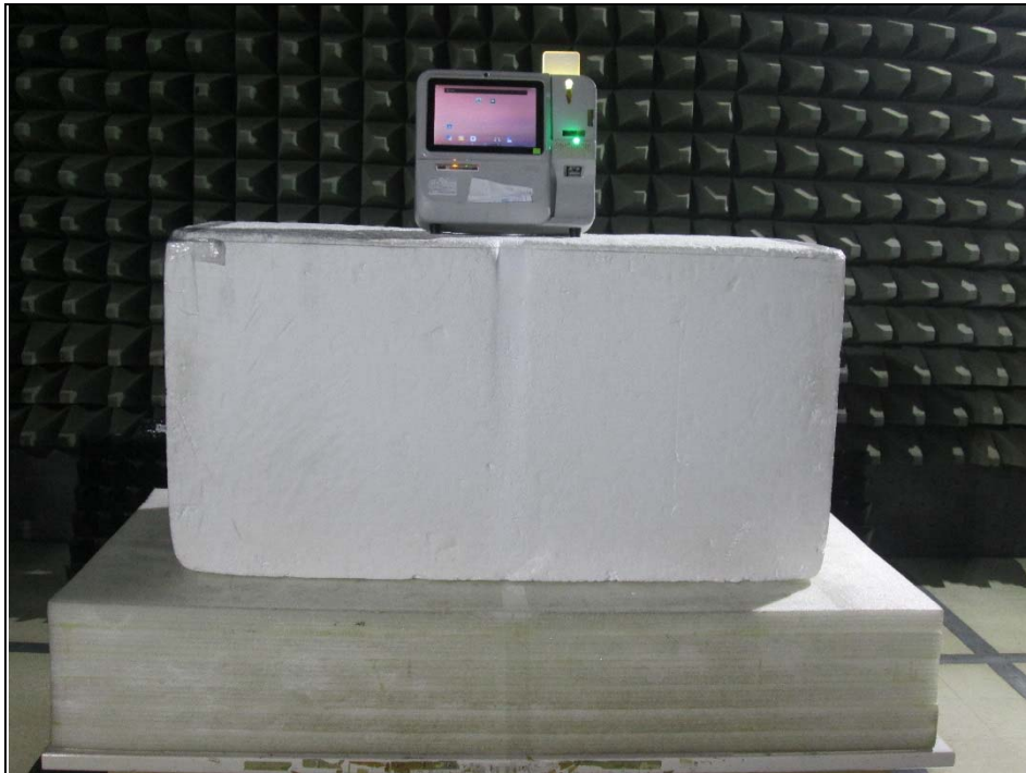
Radiated Emission Test above 1GHz
