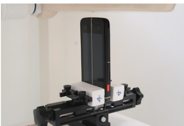
Bottom Side, Test Separation 10 mm
