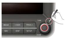
Press and hold the RESET key for about 1 second. (The use of a clip or pin is recommended when resetting the system.)
