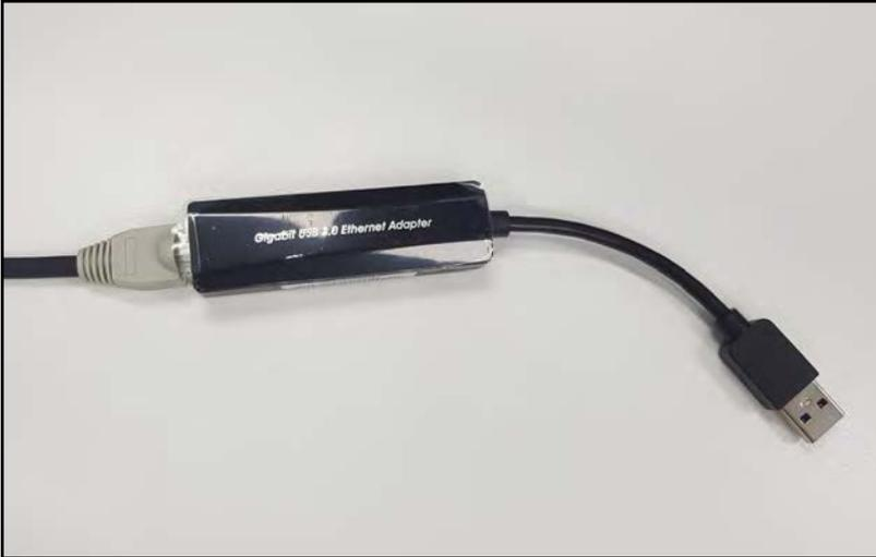
1. Plug data cable into *RJ45 to USB adaptor* (provided)
