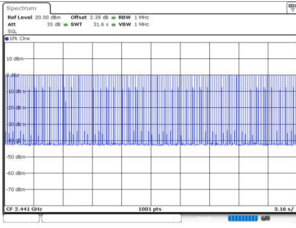
Dwell NVNT 1-DH3 2441MHz Ant1 Accumulated
