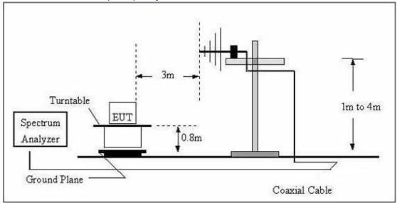
(C) Radiated Emission Test-Up Frequency Above 1GHz
