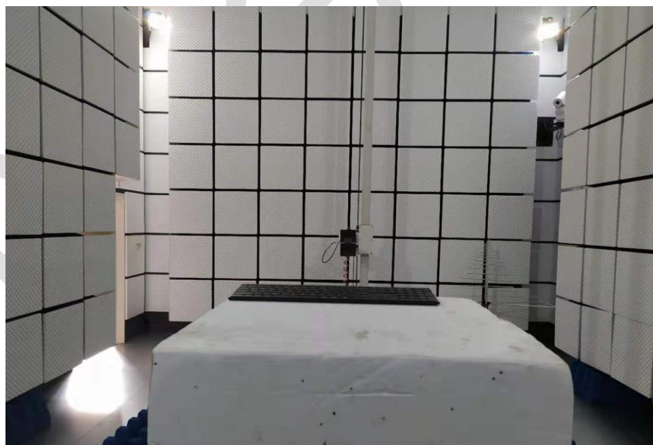
Radiated spurious emission Test Setup-3(Above 1GHz)
