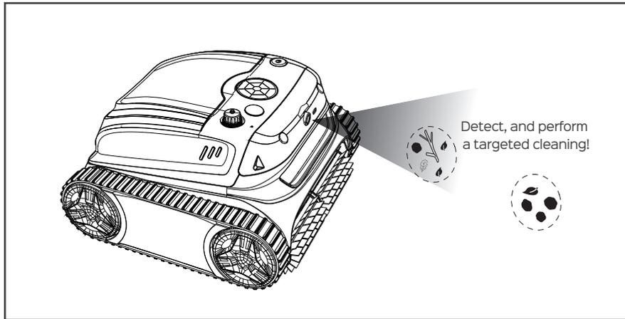
The robot needs to enrich its recognition of the dirt from the start, and it may turn on and record its floor dirt types during cleaning. It will reach its best targeted cleaning performance after one month of cleaning.
