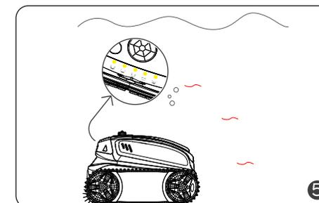
The robot will automatically move to stop by the edge of wall when finishing cleaning or battery low.
