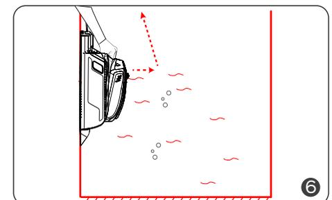
The robot will automatically move to stop by the edge of wall when finishing cleaning or battery low.
