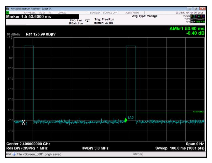
$Time\ Between\ Pulses = 53.6\ ms$   $Total\ On\ Time = 5.3\ ms$   $Total\ Duty\ Cycle = 5.30\ ms / 53.60\ ms = 9.89\%$   $The\ Maximum\ Peak\ to\ Average\ Ratio\ of\ -20\ dB\ can\ be\ used.$
