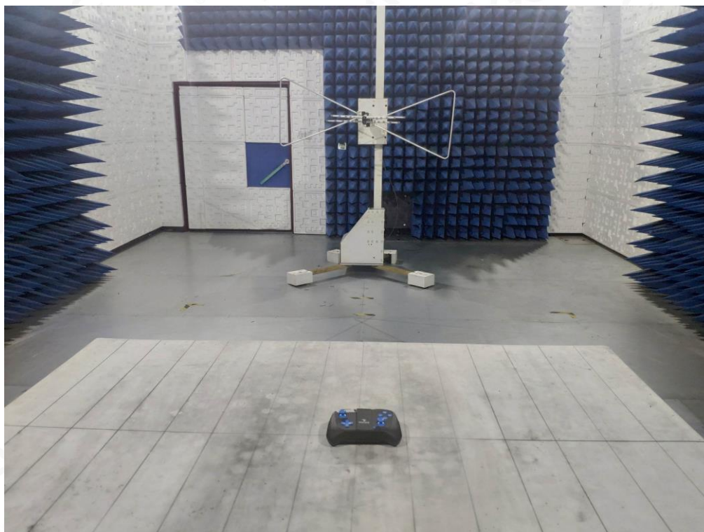
FCC RADIATED EMISSION TEST SETUP ABOVE 1GHZ
