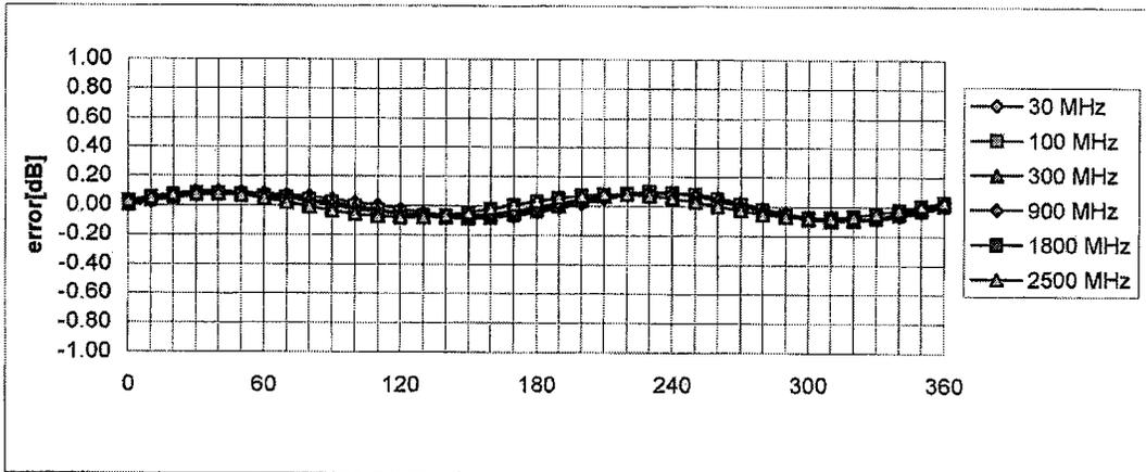
**Axial Isotropy Error  $< \pm 0.2$  dB**
