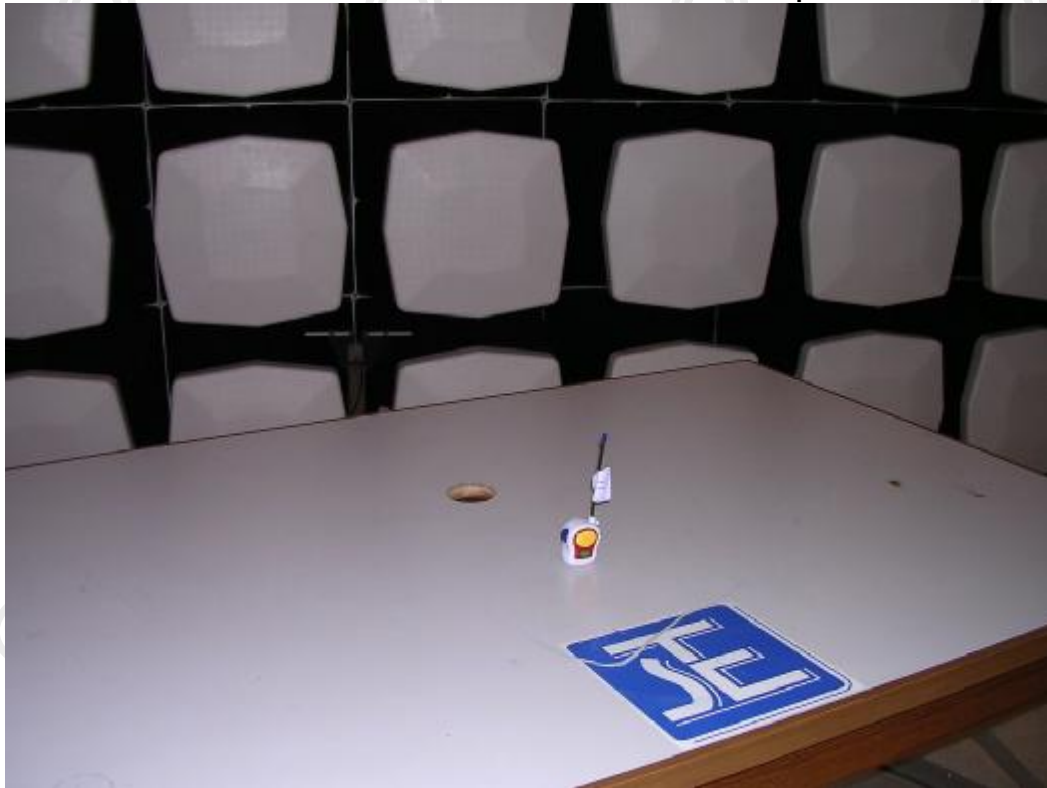
Measurement of Radiated Emission Test Set Up
