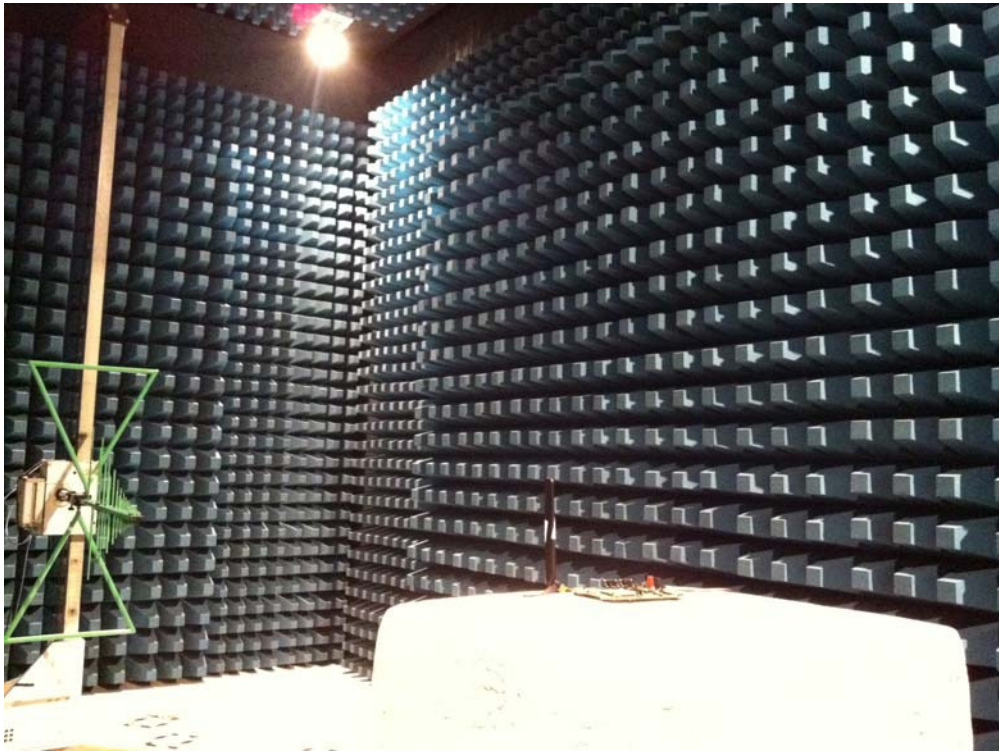
Description: ERP Test Setup
