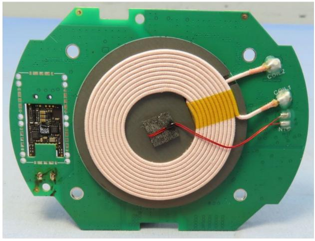
The Apple Watch charger uses a coil surrounded by a ring of magnets inside a sealed enclosure.
