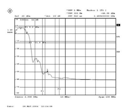
Observation: All emissions in the 100kHz bandwidth are 20dB lower than the carrier strength.
