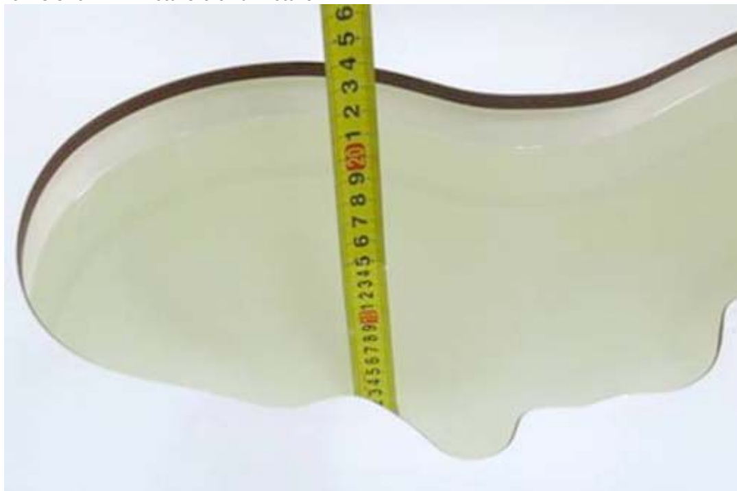
Picture 3: liquid depth in the head Phantom
