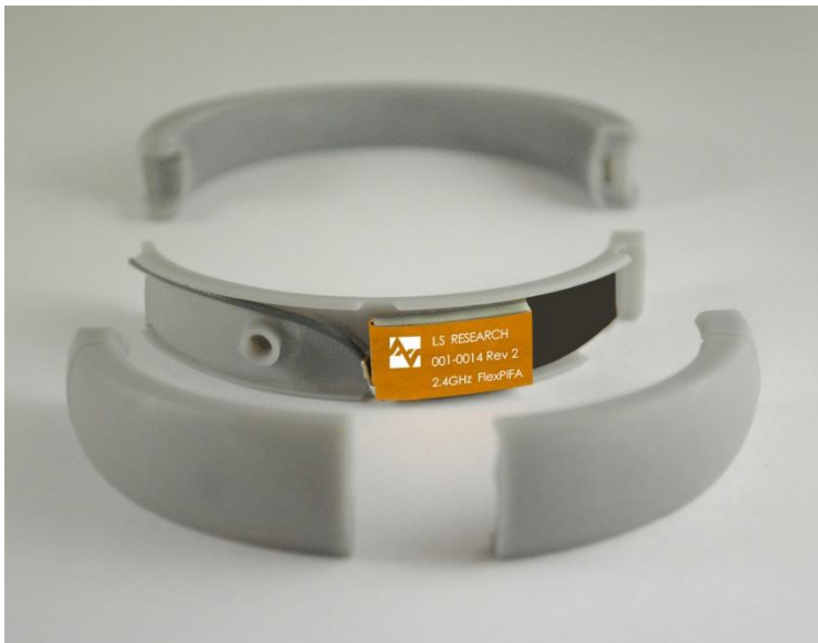
Figure 27: FlexPIFA integrated into bracelet
