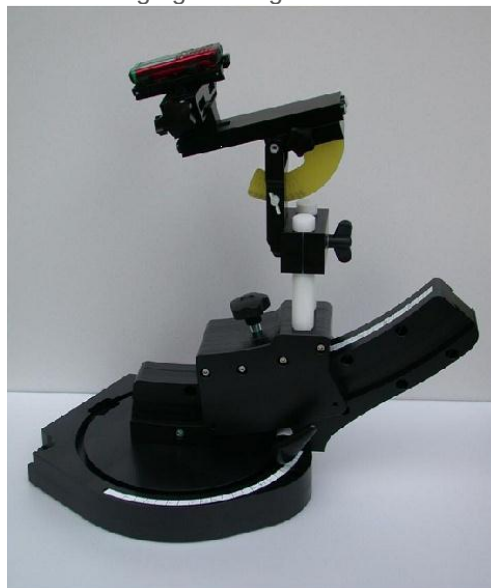
Device holder supplied by SPEAG
