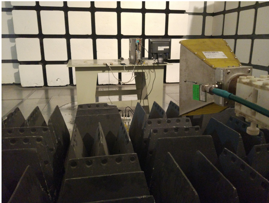
Radiated Emissions – Rear View (Above 1 GHz)
