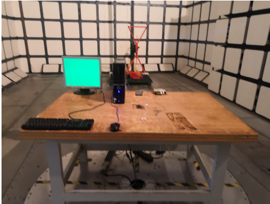
Radiated Emissions – Front View (Below 1 GHz)
