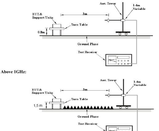
The radiated emission tests were performed in the 3 meters distance, using the setup accordance with the ANSI C63.10-2013. The specification used was the FCC 15.209, 15.247 and RSS-247 Clause 5.5, RSS-GEN Clause 8.10 limits.
