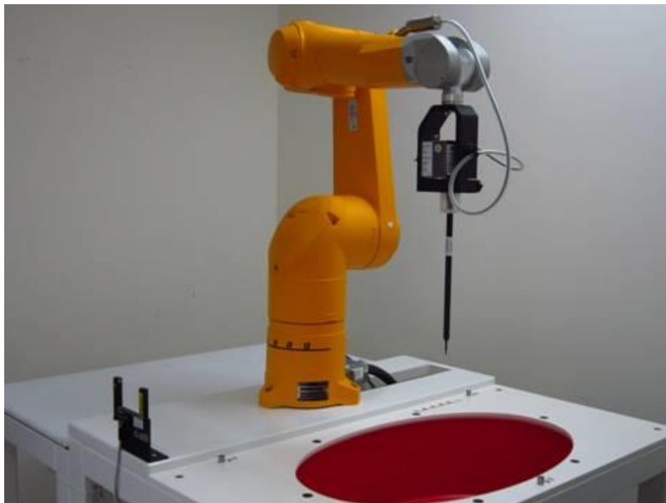
Fig.1 Photograph of the SAR measurement system
