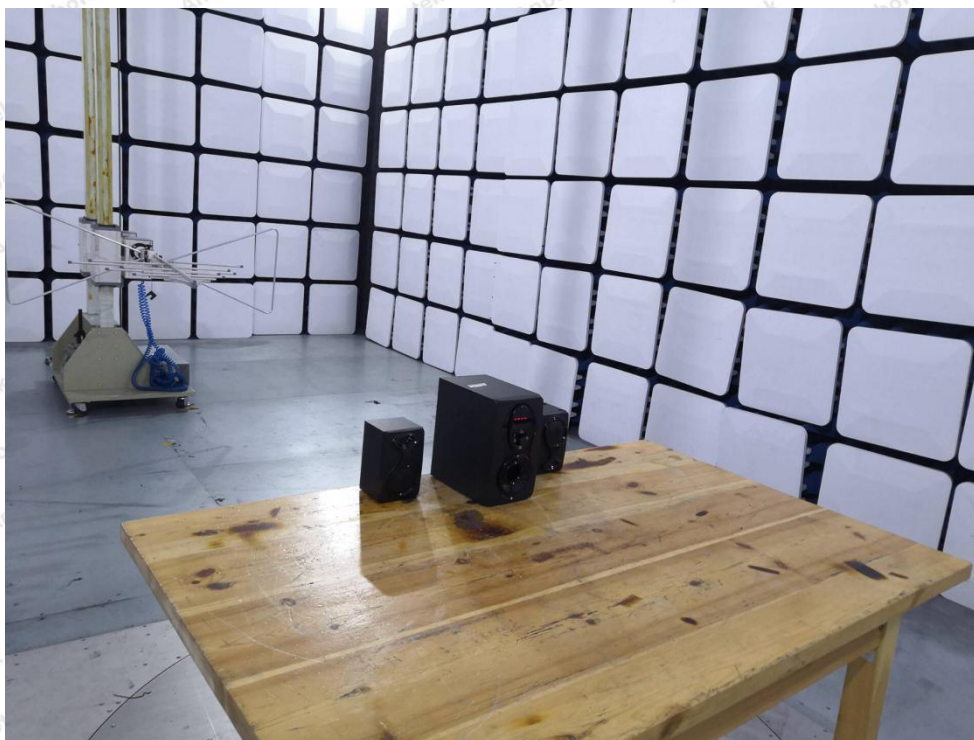
Photo of Radiation Emission Test
