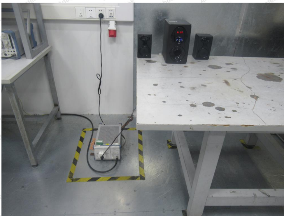
Photo of Conducted Emission Measurement
