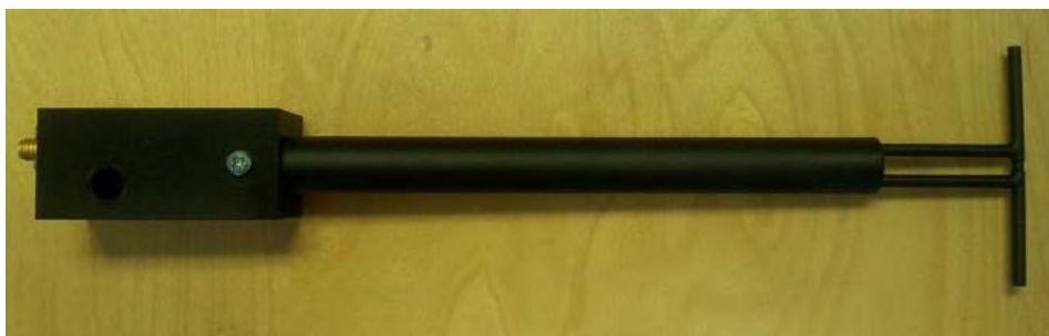
Figure 1 – MVG COMOSAR Validation Dipole
