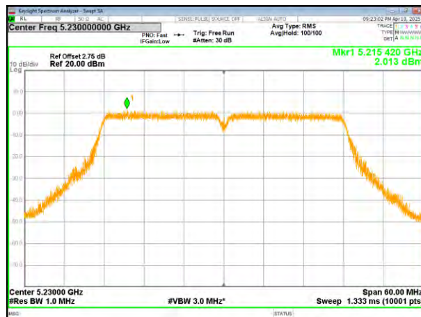
(802.11n40) PSD plot on channel 46
