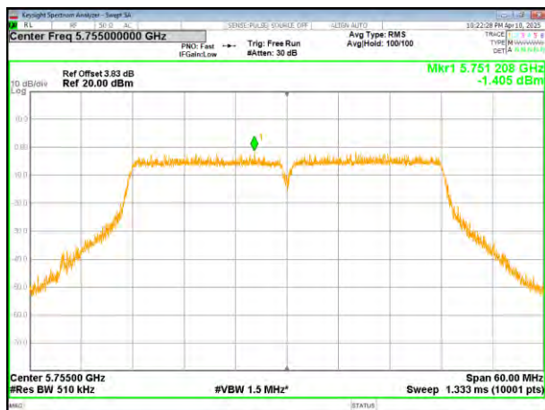
(802.11ac40) PSD plot on channel 159
