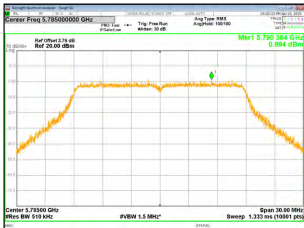
(802.11ac20) PSD plot on channel 165
