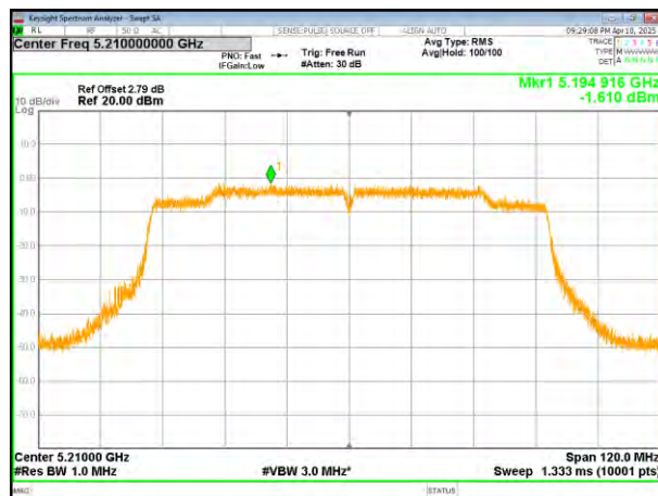
(802.11ac80) PSD plot on channel 42
