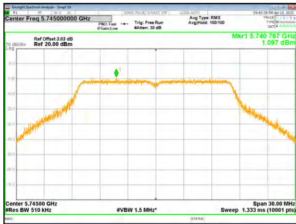
(802.11a) PSD plot on channel 157
