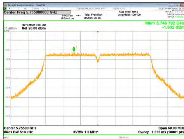
(802.11n40) PSD plot on channel 151
