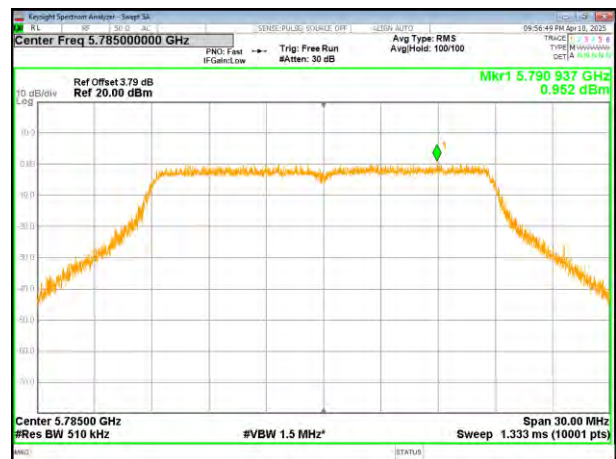
(802.11n20) PSD plot on channel 157
