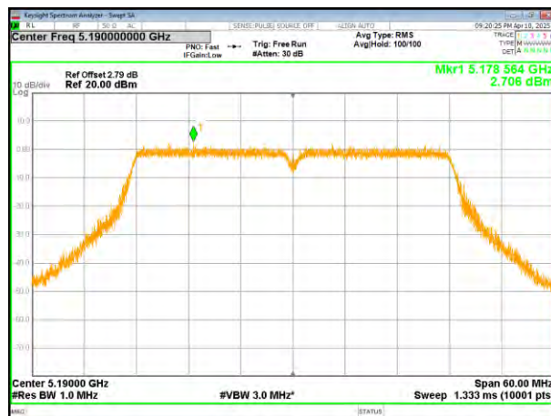
(802.11n40) PSD plot on channel 38
