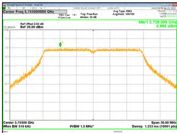
(802.11ac20) PSD plot on channel 149
