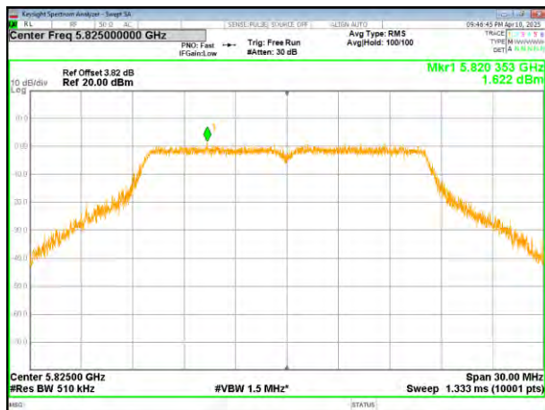
(802.11a) PSD plot on channel 165
