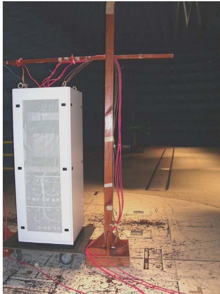
Photograph 1. Radiated Emission Limits Test Setup, 30MHz – 1GHz
