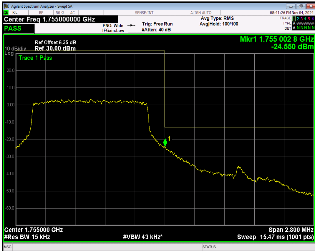
Band4 QPSK BW=3MHz Channel=19965 RB Size=15 Position=#0
