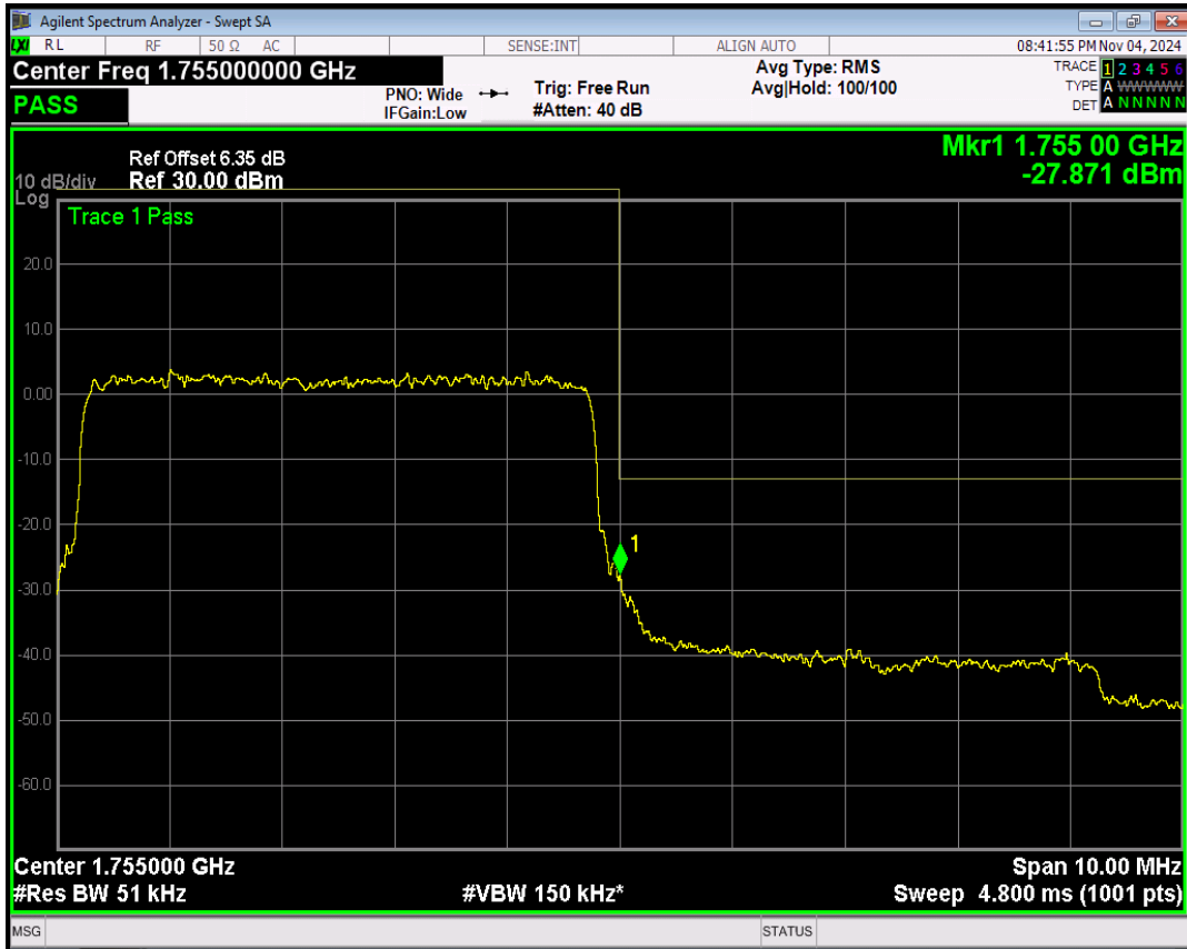
Band4 16QAM BW=5MHz Channel=20375 RB Size=25 Position=#0
