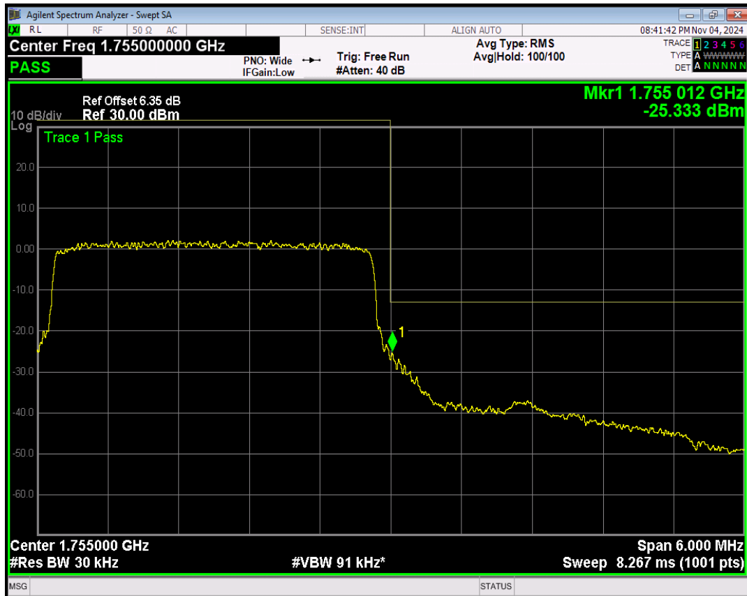
Band4 QPSK BW=5MHz Channel=19975 RB Size=25 Position=#0
