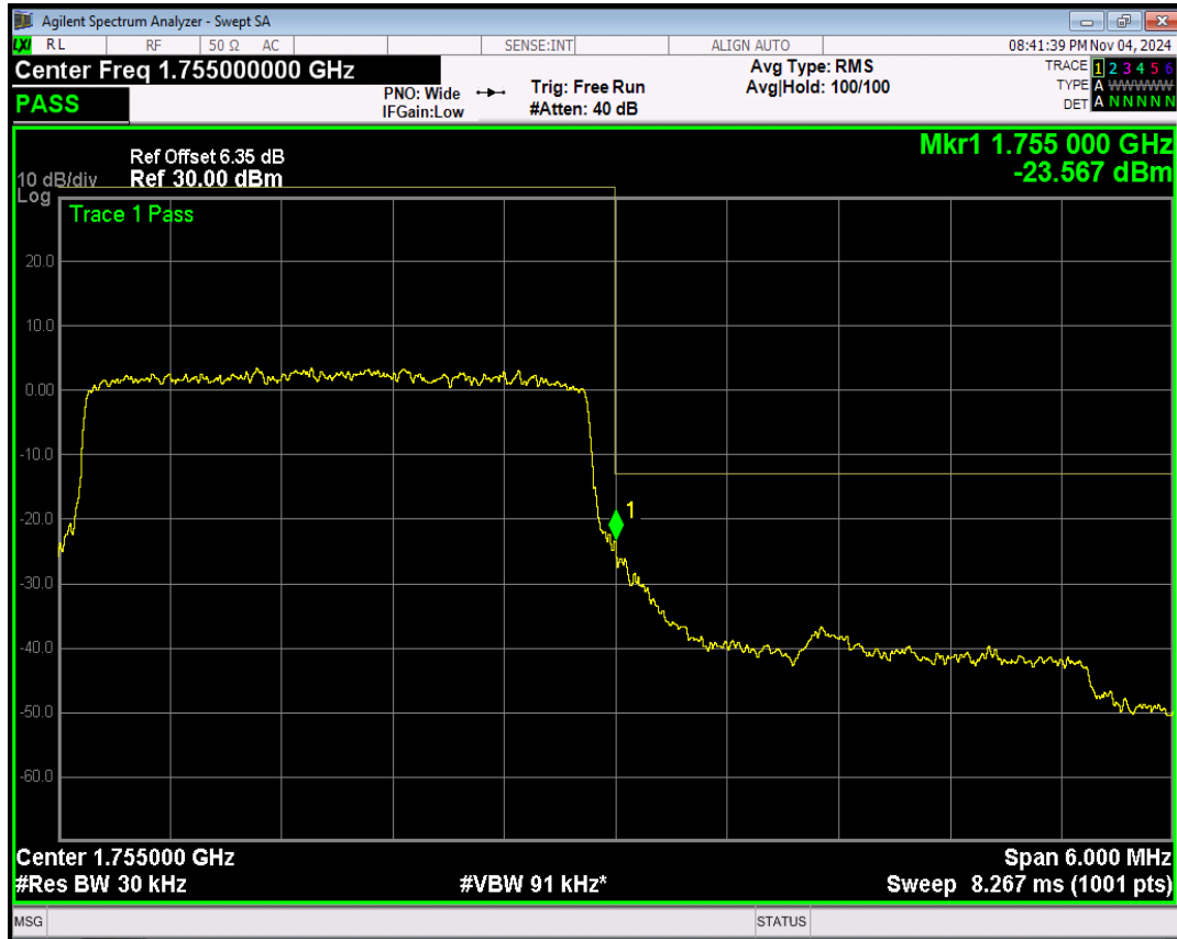
Band4 16QAM BW=3MHz Channel=20385 RB Size=15 Position=#0
