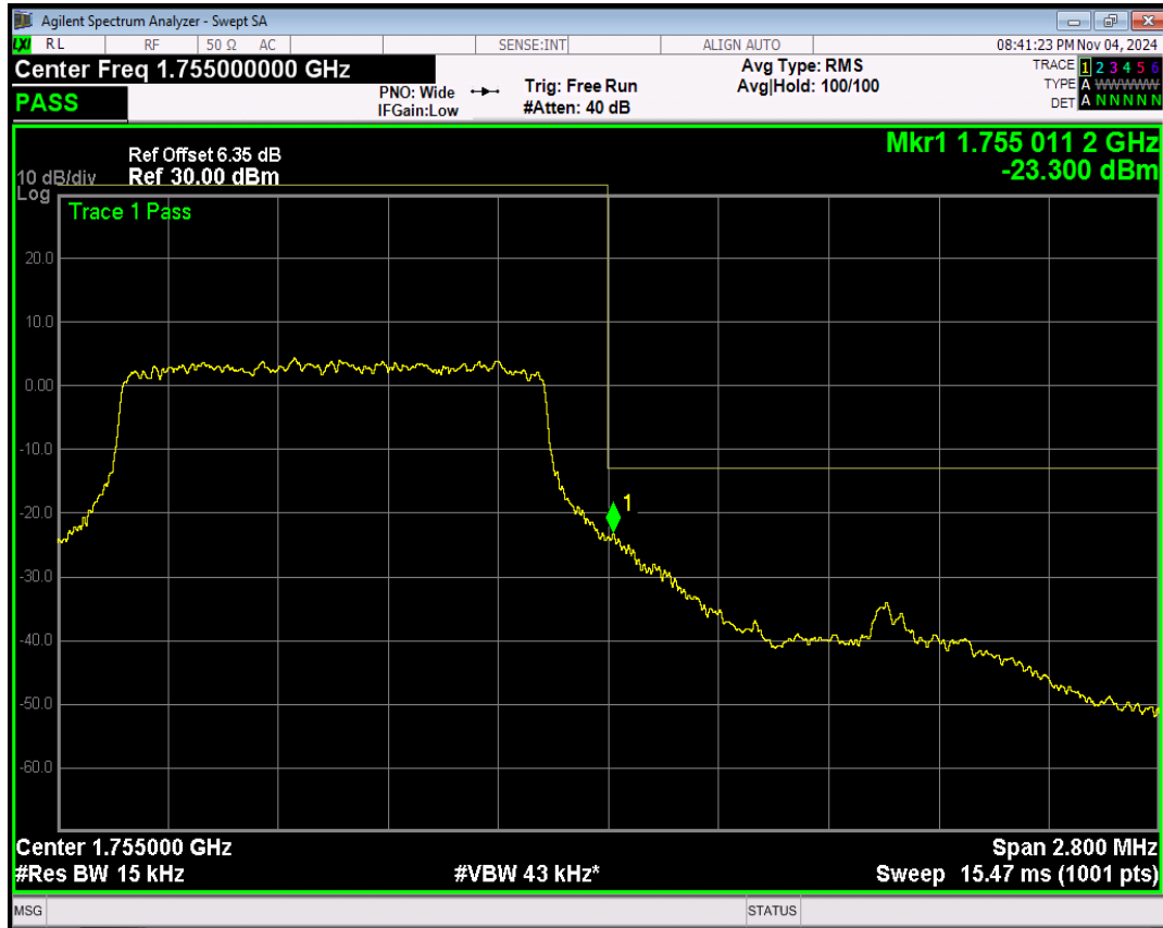
Band4 16QAM BW=1.4MHz Channel=20393 RB Size=6 Position=#0
