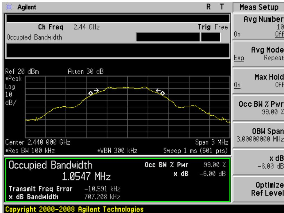
6dB Bandwidth plot on channel 39
