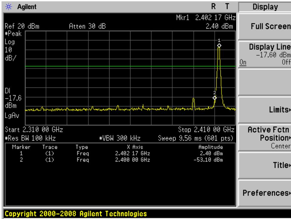
GFSK mode: Band Edge-High Channel
