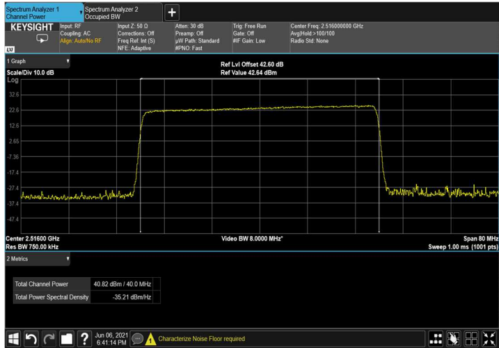
Figure 23: 64QAM 40MHz B.W.; 2516.0MHz, 15kHz
