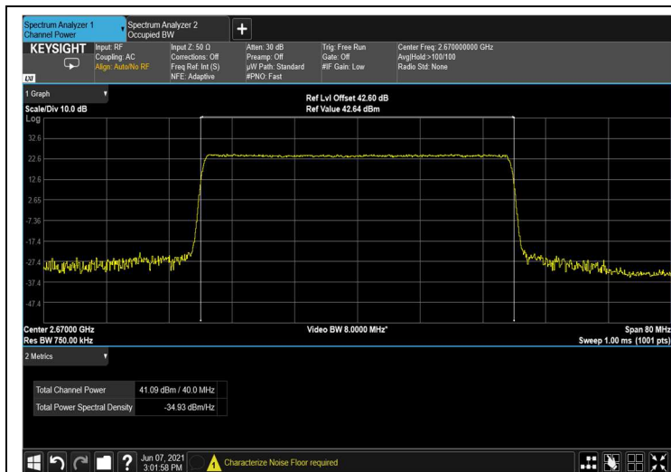
Figure 44: 256QAM 40MHz B.W.; 2670.0MHz, 15kHz
