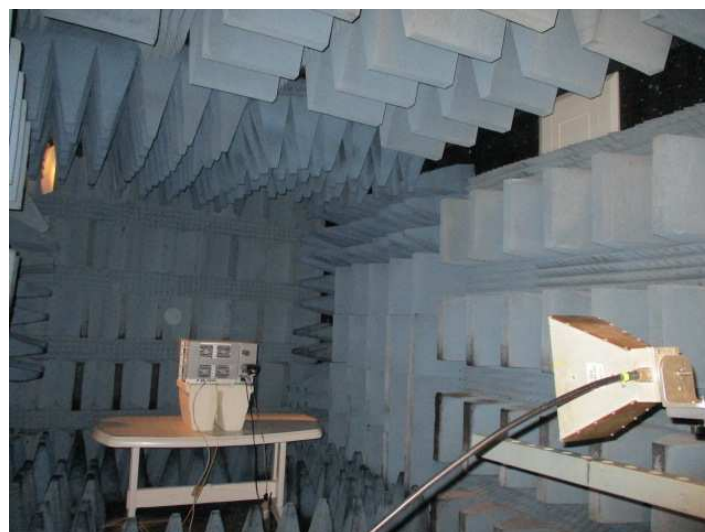
Figure 7. Radiated Emission Test 1.0 - 9.0GHz
