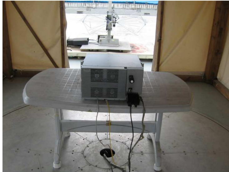
Figure 5. Radiated Emission Test 30 - 200 MHz
