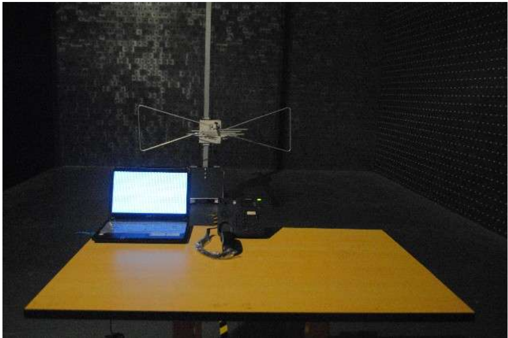
Radiated emission test view (30MHz~1GHz)
