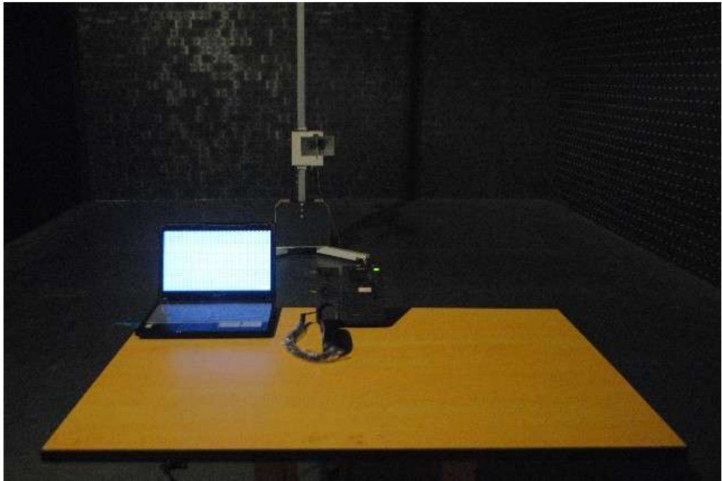
Radiated emission test view (1GHz Above)
