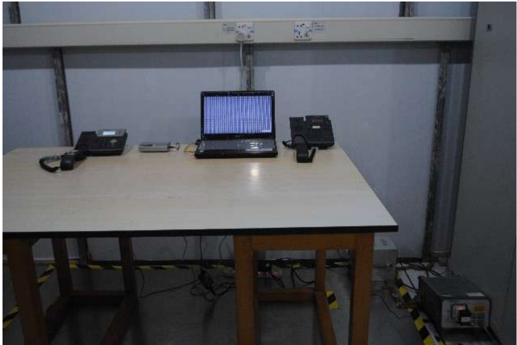
Radiated emission test view (30MHz~1GHz)
