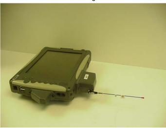
Photograph A.1-3 - Tablet PC in the Mobile Configuration Photograph A.1-4 - AirCard 580 PCMCIA Modem Card
