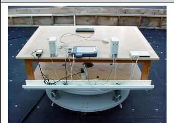
Photograph K.7-2 - Mobile DUT Configuration
