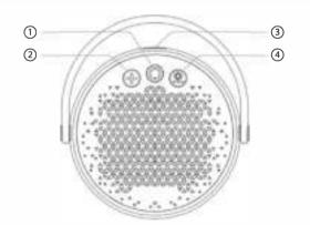
The Halo high-def stereo Bluetooth® speaker has three easy-to-use buttons on the top panel that control power, volume, and the LED light.
