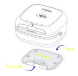
The reader can sit on the plate, but can be removed to fit any scenario.
