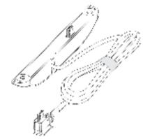
This cable with the plate attached plugs into the side of your terminal and is adhered with screws.
