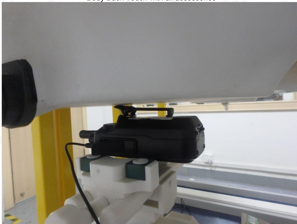
The thickness of EUT is 4.3cm
