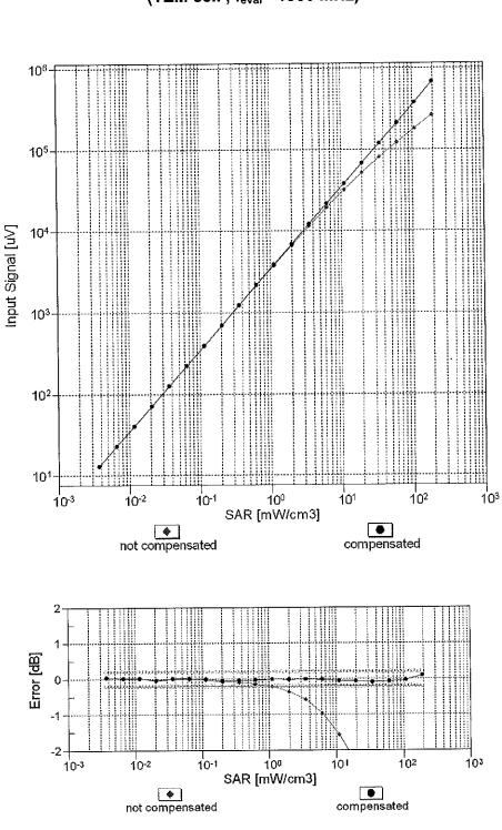
Dynamic Range f(SAR<sub>head</sub>) (TEM cell , f<sub>eval</sub>= 1900 MHz)
