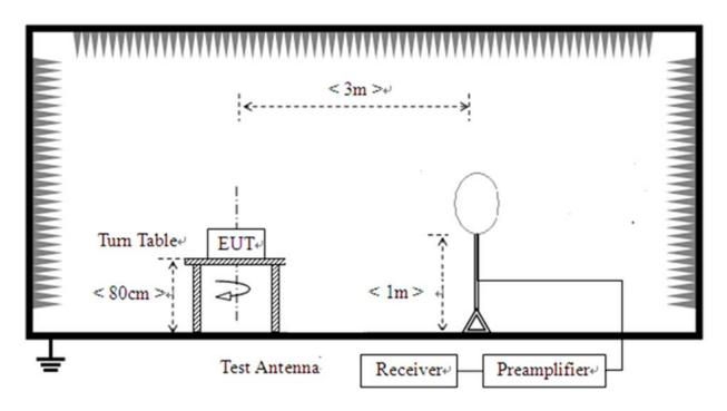
2) For radiated emissions from 30MHz to1GHz
