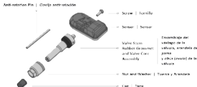
\*You must service/replace the valve when the tire is removed to uphold the sensor warranty.
