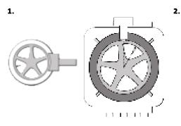
Break the bead of the tire ensuring the valve is located on Place the valve through the valve hole, ensuring the rubber When the tire is dismounted the valve must be located at 1 o'clock to the tire fitting head.
