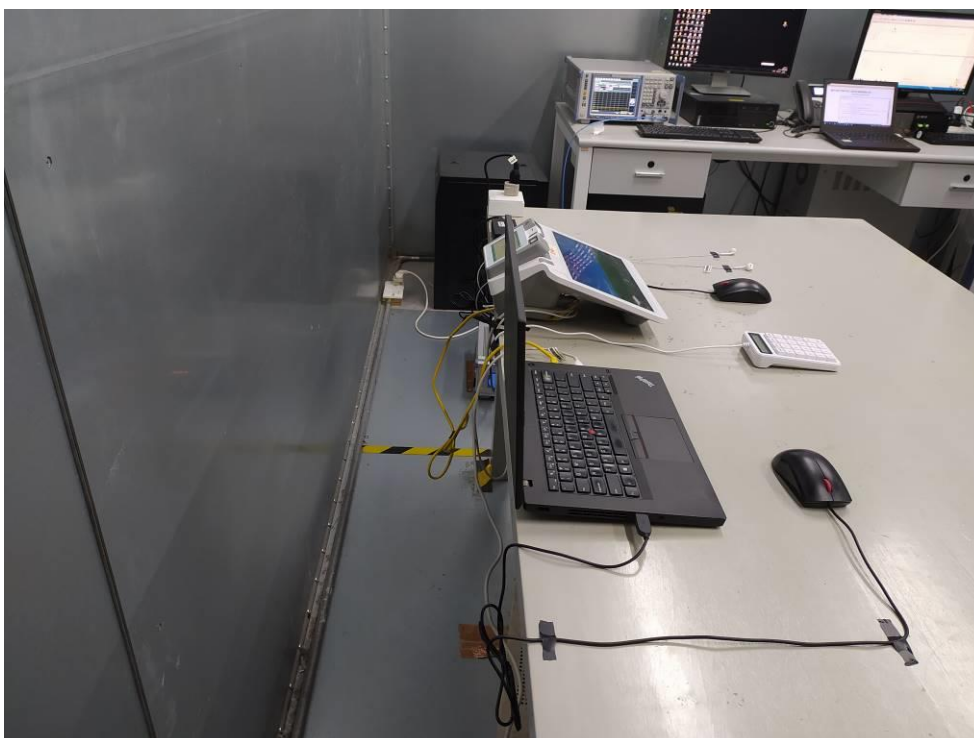
Fig. 4 Power line conducted emission setup photo
